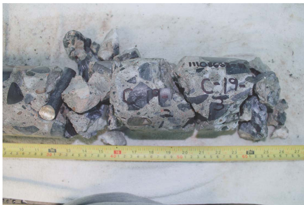
Photo 40 – Carotte C19 (profondeur 300-630 mm).
