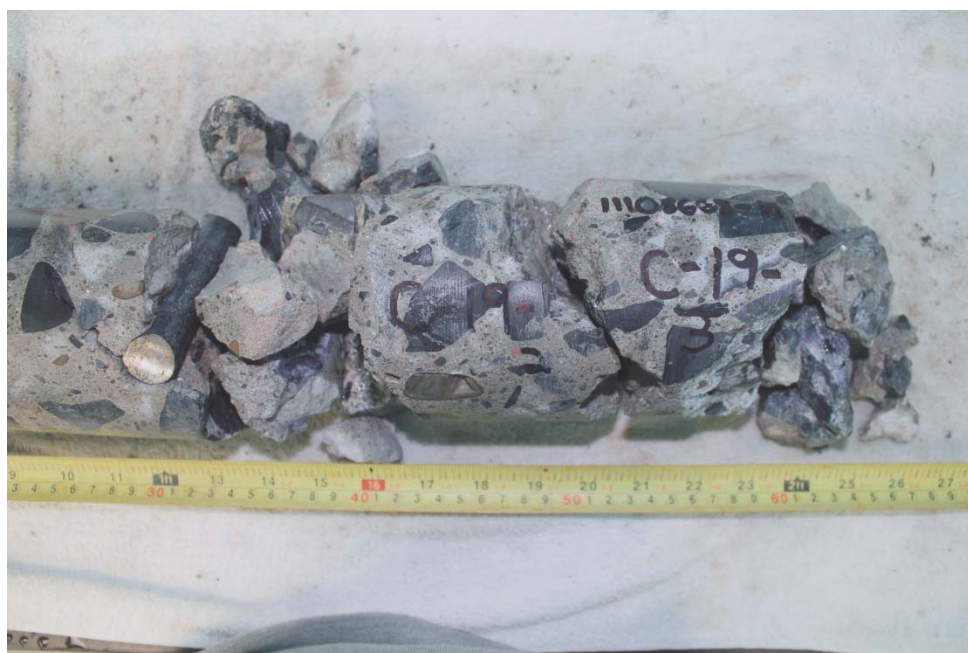
Photo 40 – Carotte C19 (profondeur 300-630 mm).
