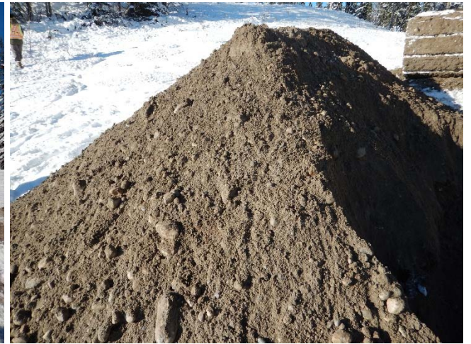
Gravel excavated from TP14-06.
