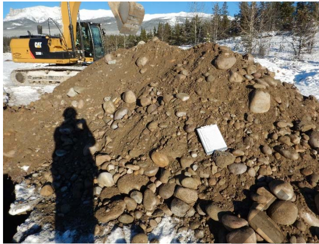
Gravel from TP14-01 excavated in existing floor.
