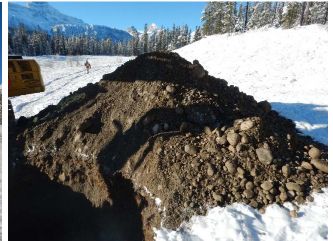
Gravel excavated from TP14-06.
