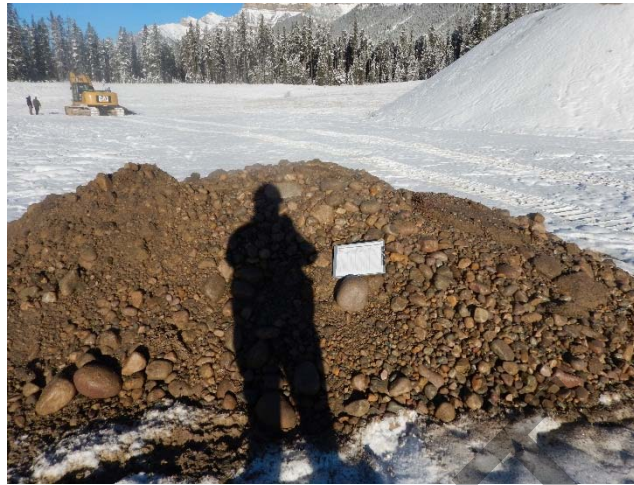
Gravel excavated from TP14-01.
