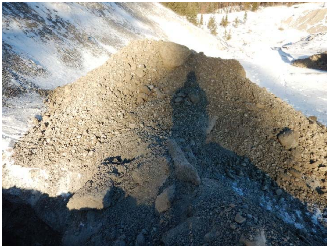
Excavated gravel from TP14-01. Gravel had clay coating.
