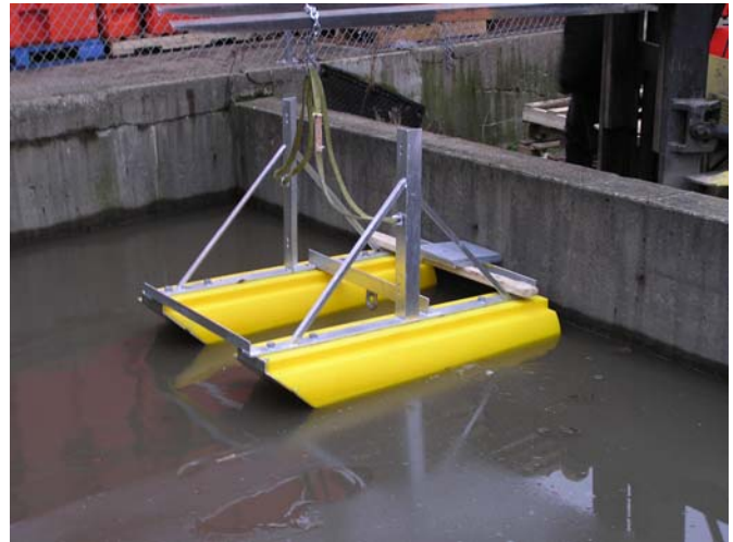
Float Test AFTER adding ballast
