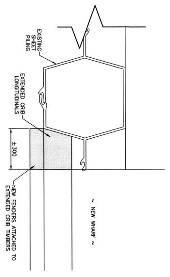
**FENDERING AT INTERFACE WITH SHEET PILE WALL**
