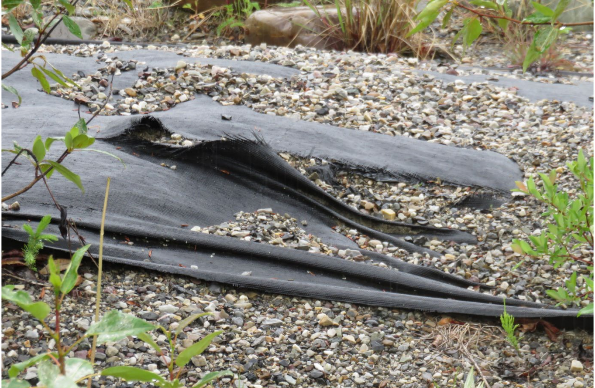
Photograph 7: Close up of suspect (woven) liner.
