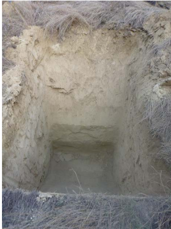
Photo 28: TP10 – Excavated test pit up to 3 m.
