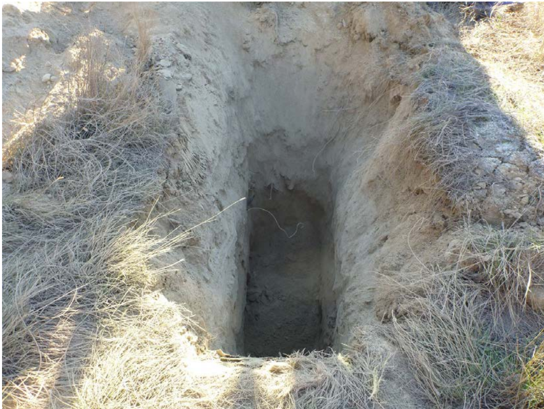
Photo 4: TP1 – excavated to 3 m. No debris but soil is disturbed/fill material.
