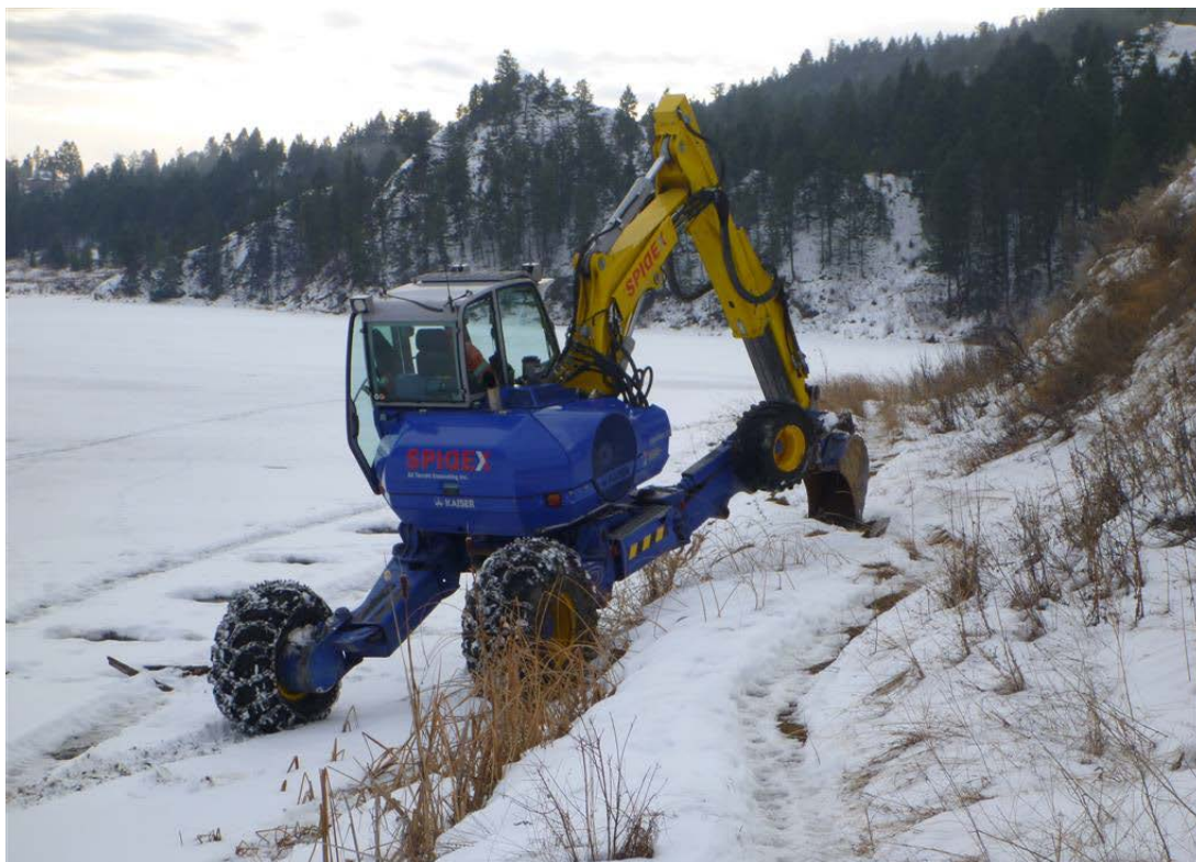
Photo 64: Due to very thin ice condition, spider hoe moved out of marsh by trail.
