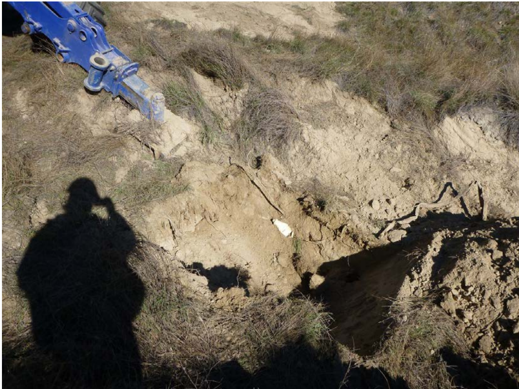
Photo 14: TP7 – debris observed at 0.5 m.
