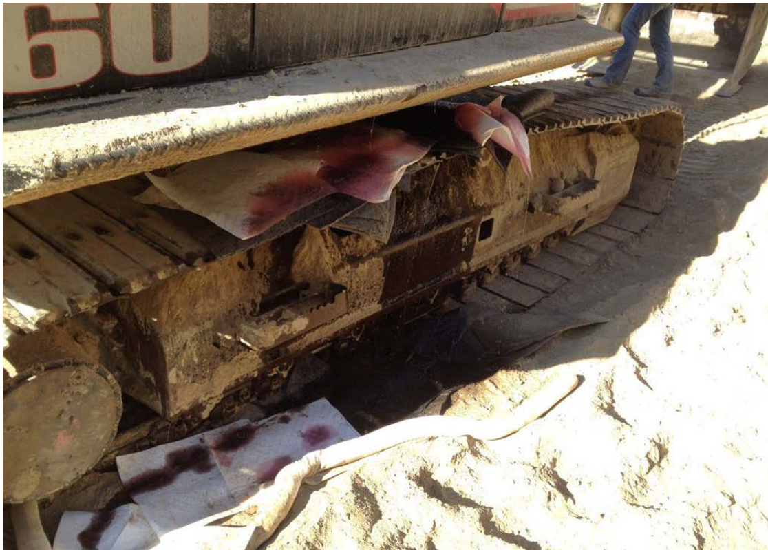
Photo 85: Loss of diesel fuel due to damage to fuel shut off valve.
