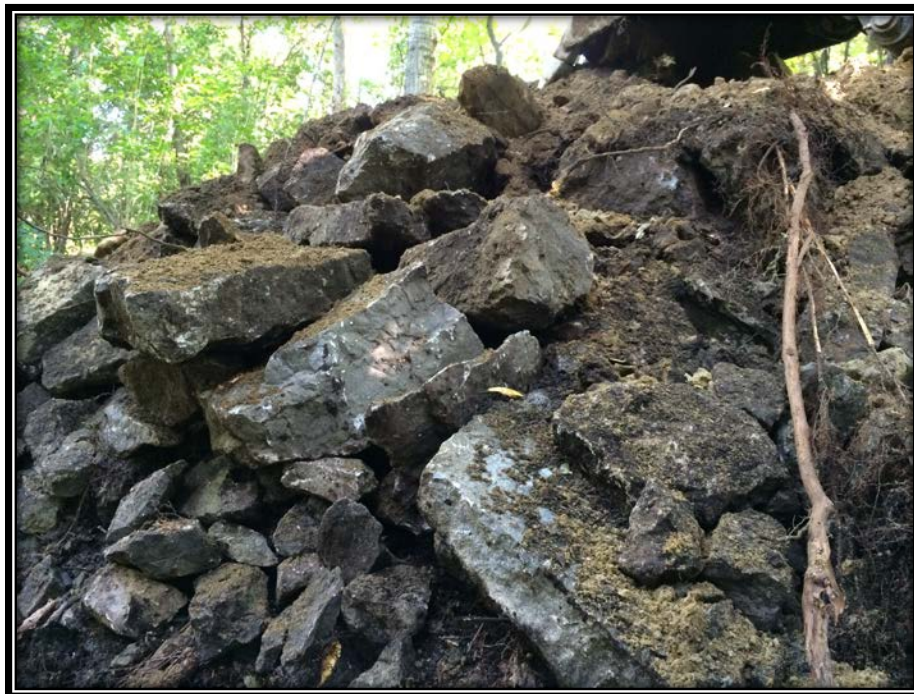
Figure 6 –TP3-N, spoils from excavation (fill materials)
