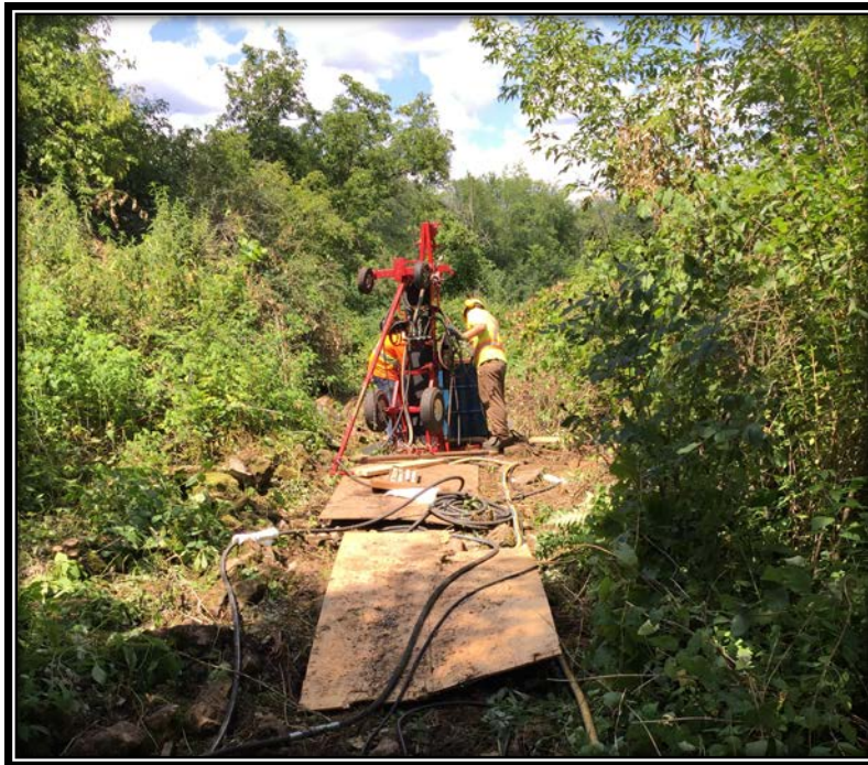
Figure 3 – 'Beaver' man-portable rig during drilling operations (July 30-2015)
