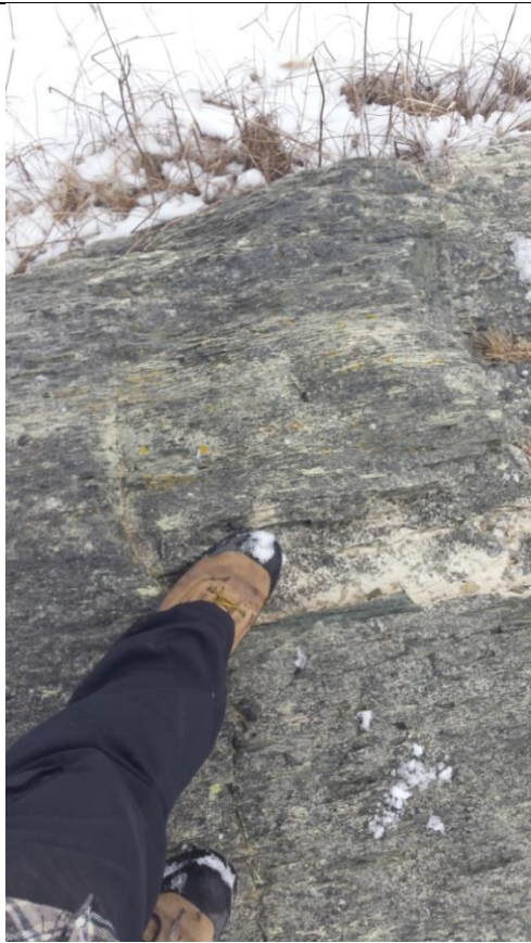
Photo 25: Outcrop H located ~ 25 m NE of approximate location of Turbine 14-05 exhibiting close spaced jointing and cleavage planes.
