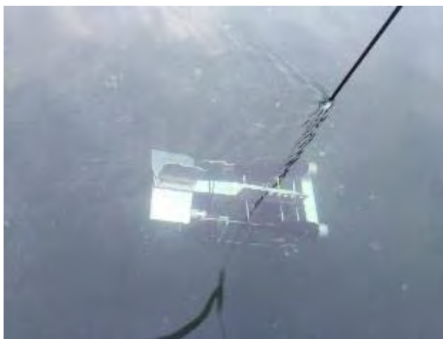
Photograph 2: Towed video camera during survey – Jan 26, 2016
