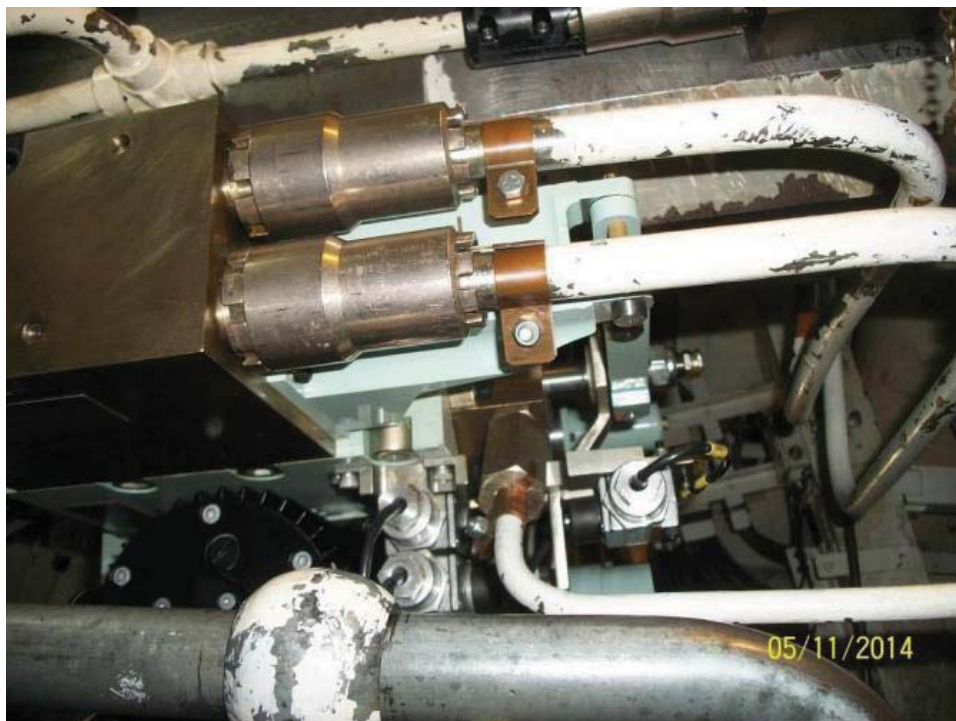
Figure 22: After Hydroplane RSU Front End Hydraulic Connections
