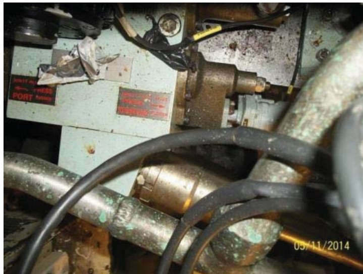
Figure 24: Rudder RSU Hydraulic Connections Top View
