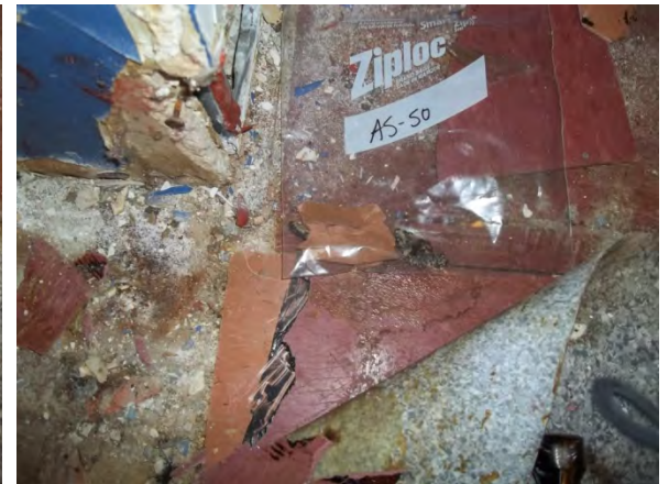
Photo 51: View of vinyl floor tile and mastic sample AS-50.
