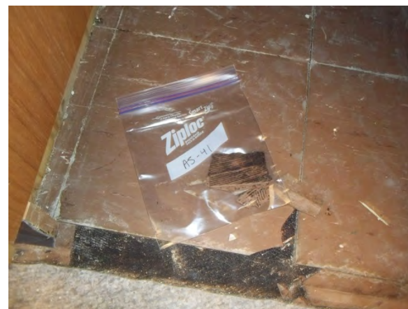
Photo 42: View of vinyl floor tile and mastic sample AS-41.
