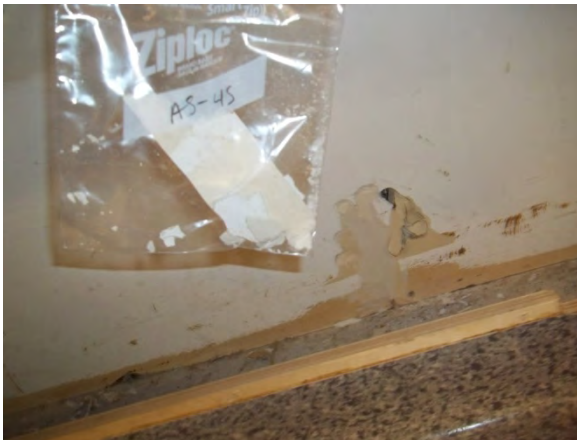
Photo 46: View of drywall joint compound sample AS-45.
