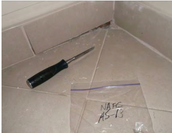
Photo 14: View of ceramic tile grout sample AS-13.
