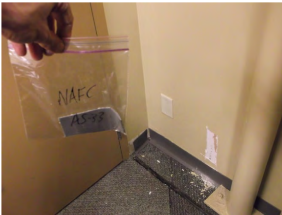
Photo 34: View of baseboard and mastic sample AS-33.
