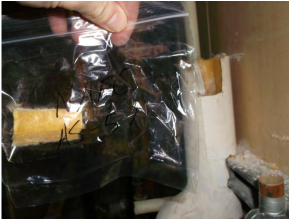
Photo 58: View of straight-run pipe insulation sample AS-57.
