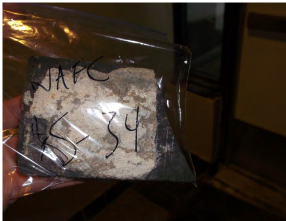
Photo 35: View of ceramic tile and grout sample AS-34.
