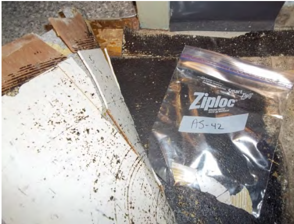
Photo 43: View of vinyl floor tile and mastic sample AS-42.
