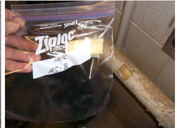
Photo 9: View of straight-run pipe insulation sample AS-08.
