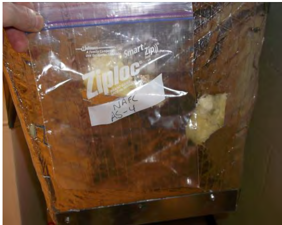
Photo 5: View of duct insulation sample AS-04.
