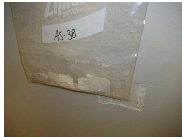
Photo 39: View of drywall joint compound sample AS-38.
