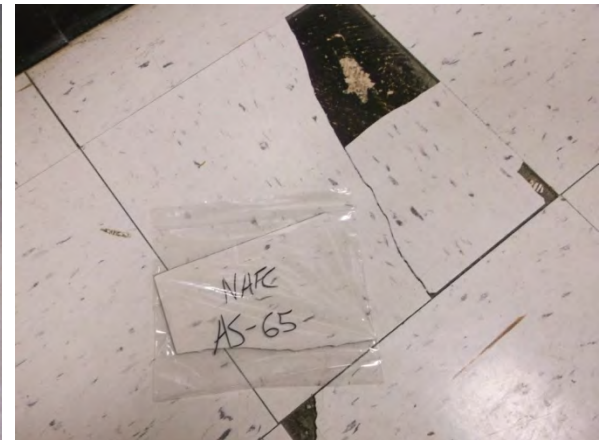
Photo 66: View of vinyl floor tile and mastic sample AS-65.
