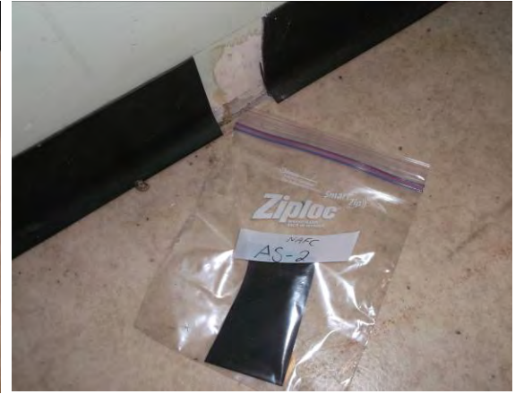
Photo 3: View of baseboard and mastic sample AS-02.
