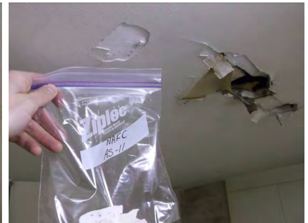
Photo 12: View of drywall joint compound sample AS-11.
