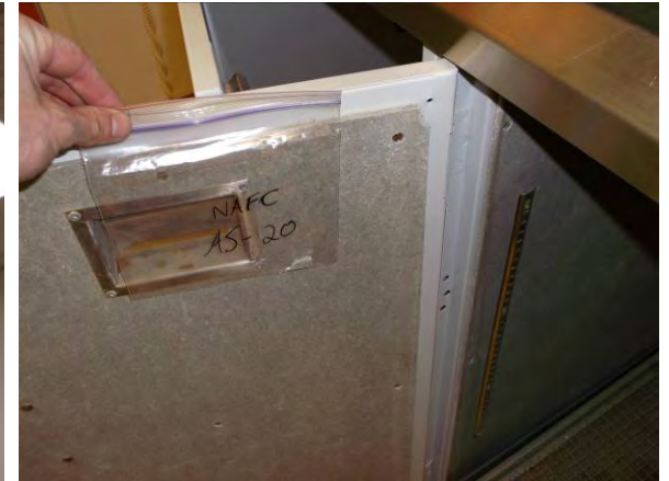
Photo 21: View of cement board (transite) sample AS-20.
