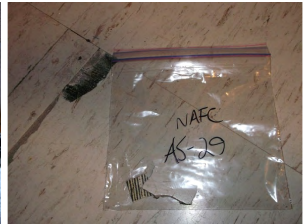
Photo 30: View of vinyl floor tile and mastic sample AS-29.
