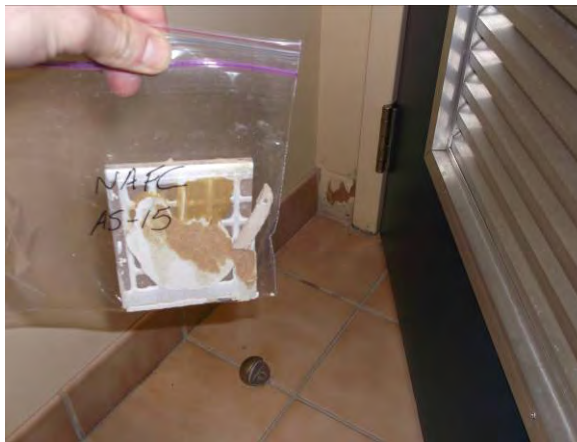
Photo 16: View of ceramic tile and grout sample AS-15.
