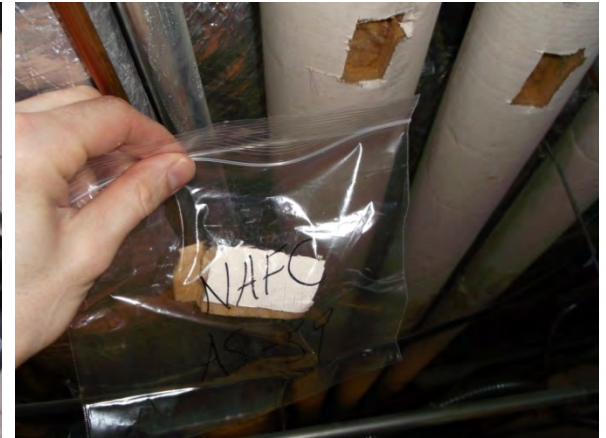
Photo 60: View of straight-run pipe insulation sample AS-59.
