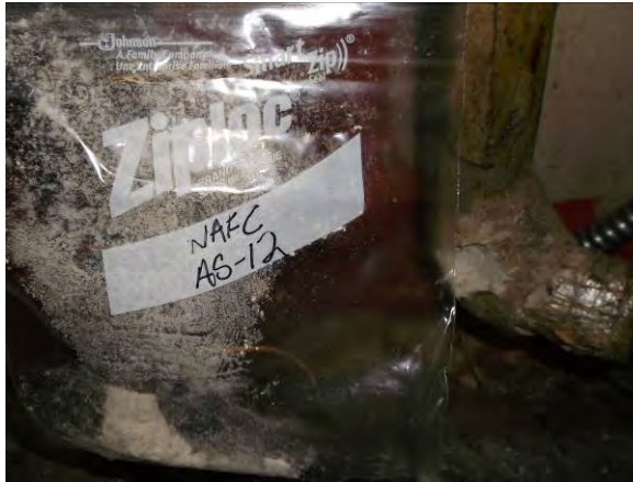
Photo 13: View of pipe elbow parging sample AS-12.
