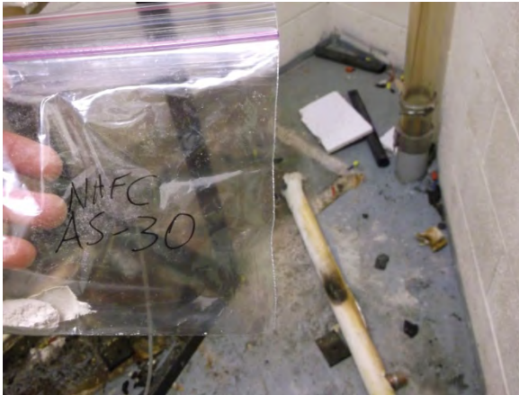
Photo 31: View of pipe elbow parging sample AS-30.
