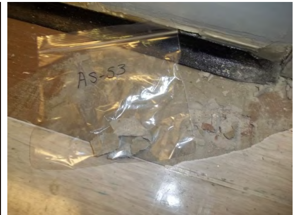
Photo 54: View of floor levelling compound sample AS-53.
