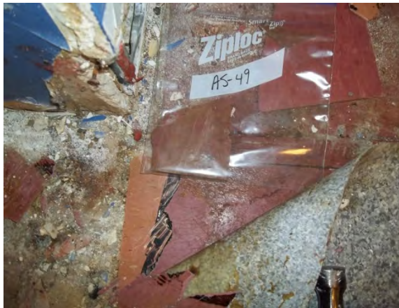
Photo 50: View of vinyl floor tile and mastic sample AS-49.
