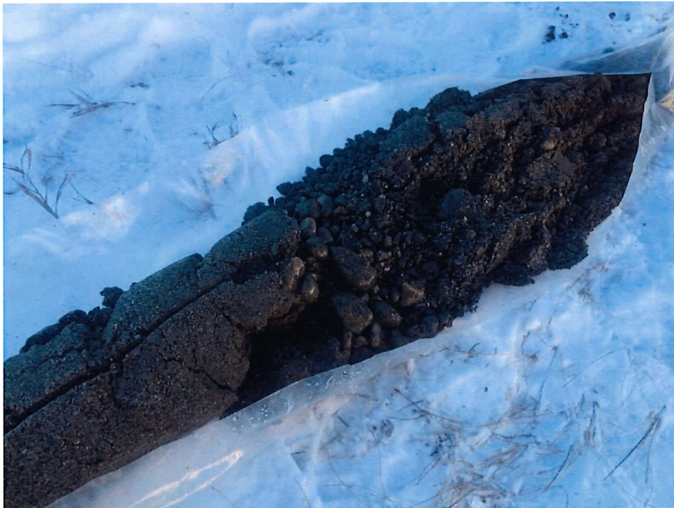
Photograph 3: AEC 6 Sample core of 6-BH15-29, showing coarse gravel and sand layers.
