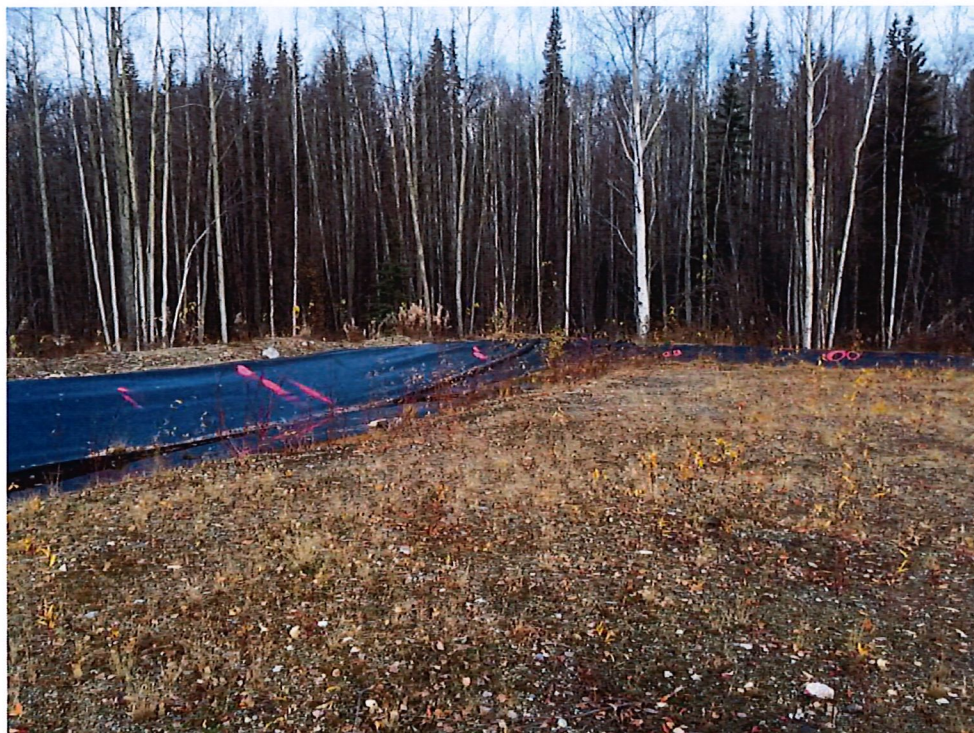
Photograph 12: Small to medium size liner perforations along LTF berm.
