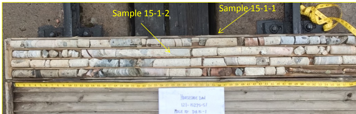
DH15-1 Box 1 of 2. Concrete core of 30 mm size. Void at bottom of hole for last 30 cm (no core retrieved).
