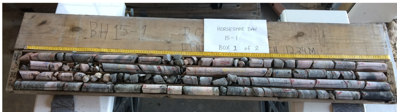
DH15-1 Box 2 of 2 showing rock core from 5.7 m to 11.7 m. Feldspathic rich layered intrusive of moderate metamorphism with gneissic texture at 45 degrees to core axis. Medium to coarse grained with poorly defined foliation.
