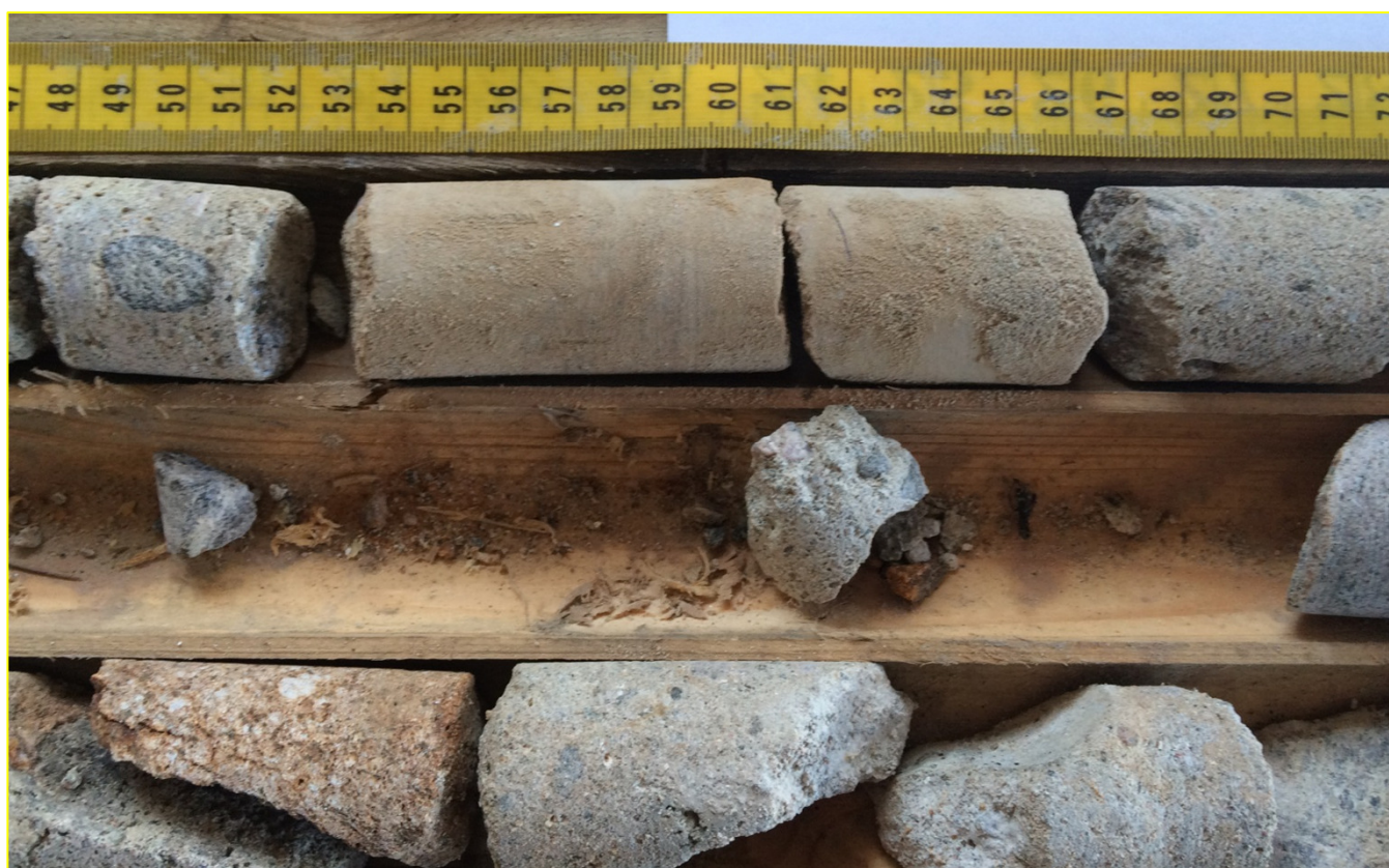
DH15-3 detail showing very friable concrete and poor recovery sections.
