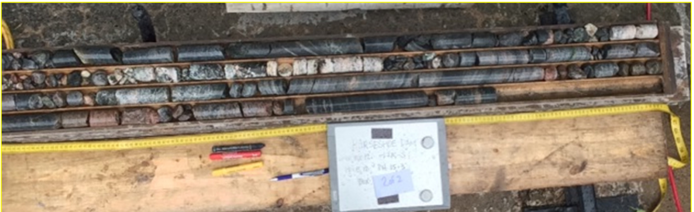
DH15-2 Box 2 of 2: Mostly dark banded rock units with some pink to buff coloured feldspathic units.
