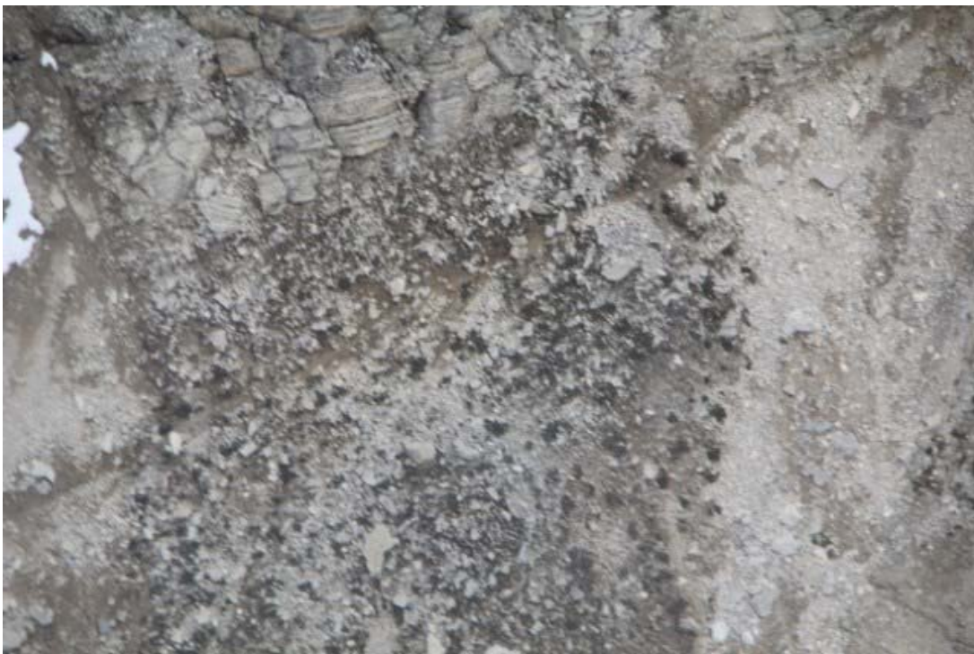
Photo 27: Slide path 4 – loose surficial materials appear to include a silt/sand matrix
