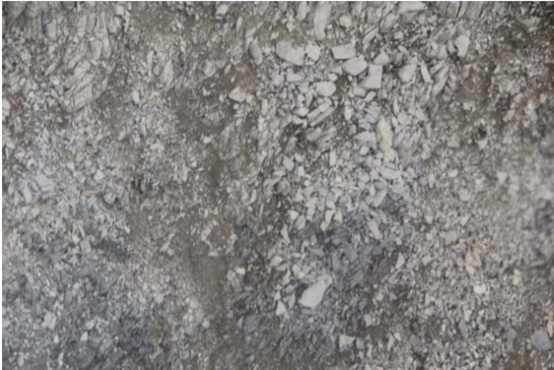
Photo 24: Slide path 4 – loose surficial materials appear to include a silt/sand matrix
