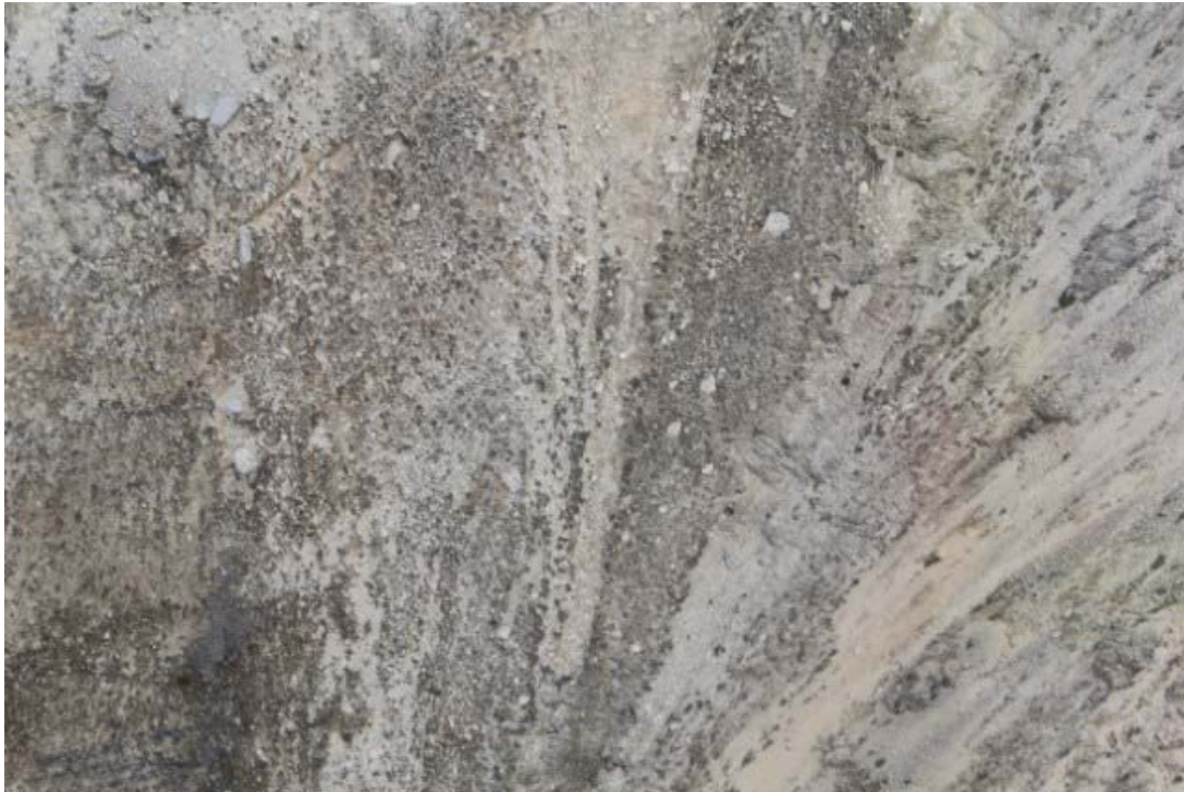
Photo 28: Slide path 4 – loose surficial materials appear to include a silt/sand matrix
