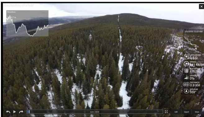
KM 0-8.3: Generally well defined cut line through coniferous forest. Trees of varying height to be cleared. Lower brush was generally masked by the lingering snow.
