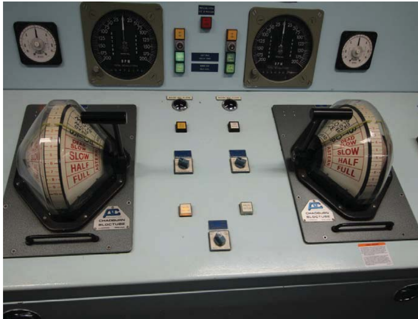
10.6 Figure 6 MCR telegraphs, RPM and transfer control
