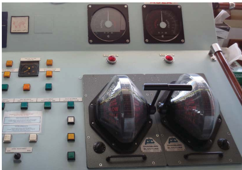
10.7 Figure 7 Bridge telegraph and RPM gauge setup
