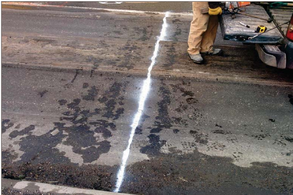
Photo 2: View of the lane cross-section surveyed (Figure 2). Four cores were taken along the white line – two in the wheel paths, one between the wheel paths, and one at the far edge of the lane.
