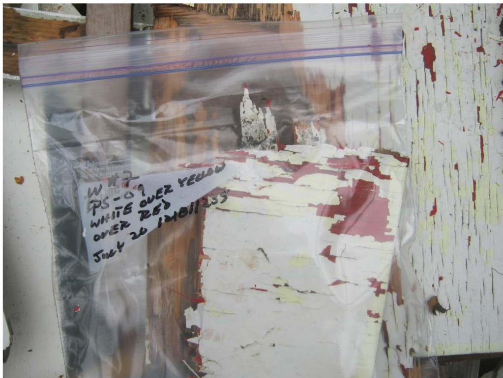
PHOTO 12: View of paint sample C-PS-09 (white over yellow over red paint on wood substrate) found to be lead-containing. This paint sample was obtained from a wood door of the partially demolished building WKS 7 located at the Chignecto South Campground.
