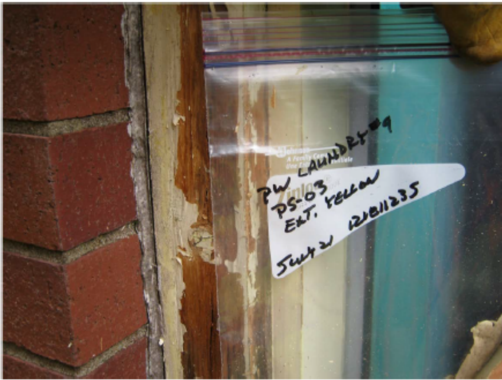
PHOTO 15: View of location of paint sample PW-PS-03 (yellow paint on wood substrate) found to be lead-containing. This yellow colour paint was observed on the exterior doors, wood panels, and masonry of building L9 located at the Point Wolfe Campground.
