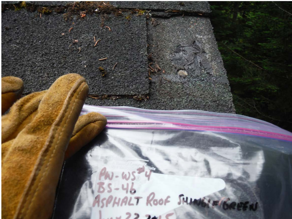
PHOTO 11: View of sample PW-BS-46 (green asphalt shingle) obtained from the roof of building WS 4 . This shingle sample was found to 3.1% Chrysotile asbestos .
