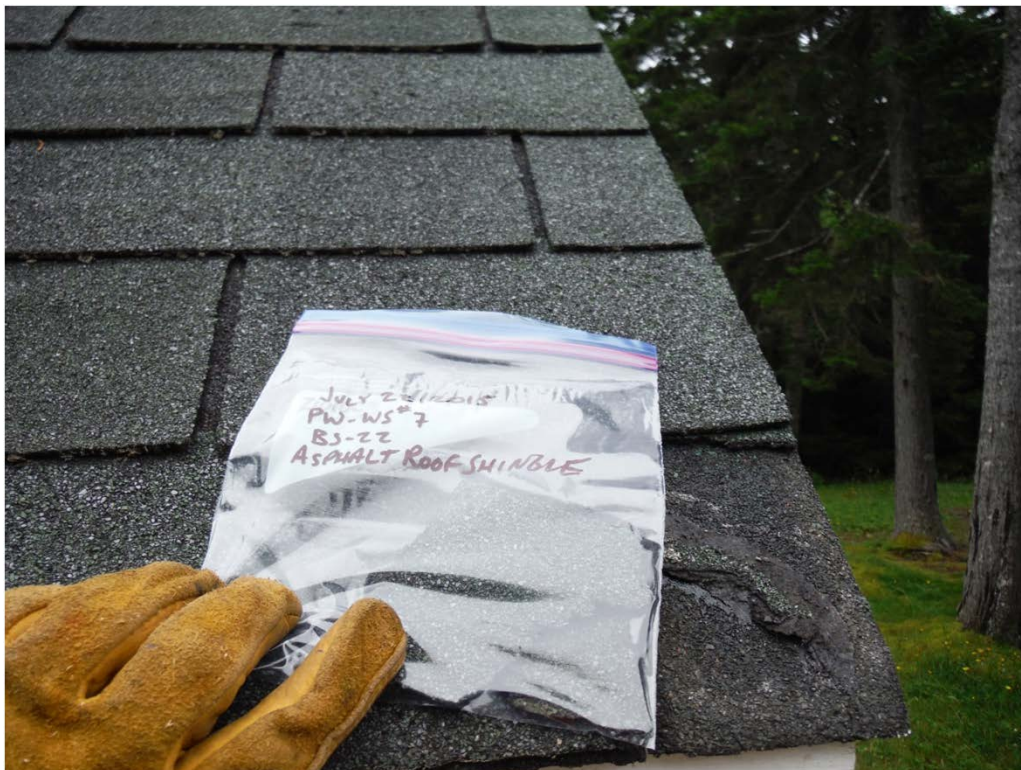
PHOTO 10: View of sample PW-BS-22 (green asphalt shingle) obtained from the roof of building WS 7 located in the Point Wolfe Campground. This shingle sample was found to contain 0.55% Chrysotile asbestos .
