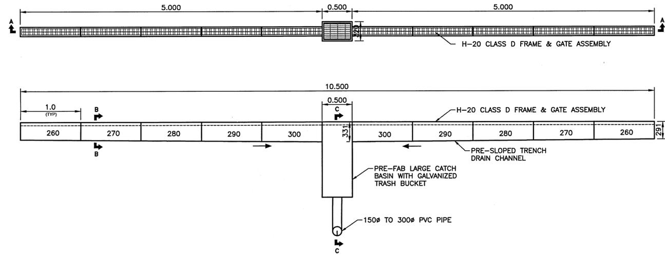
TRENCH DRAIN DETAIL & SECTION A-A
