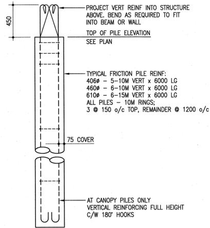
**TYPICAL FRICTION PILE DETAIL**
