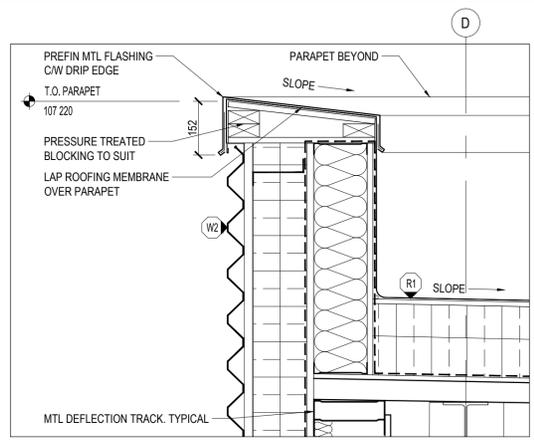
16 TYPICAL PARAPET SECTION DETAIL
