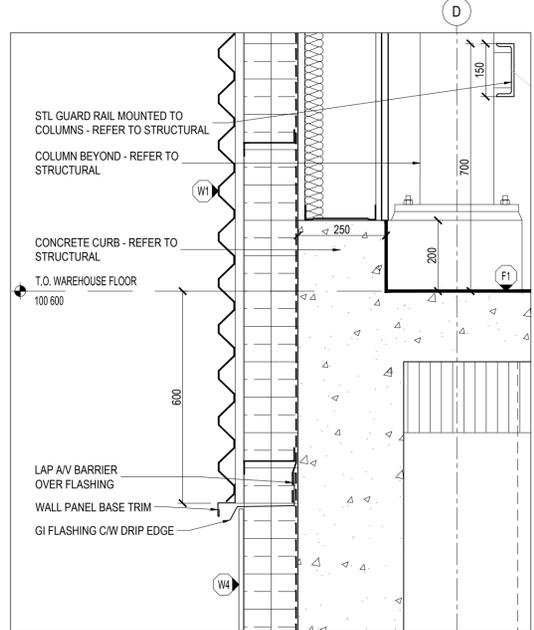
13 TYPICAL GRADE BEAM AT FLOOR SECTION DETAIL
