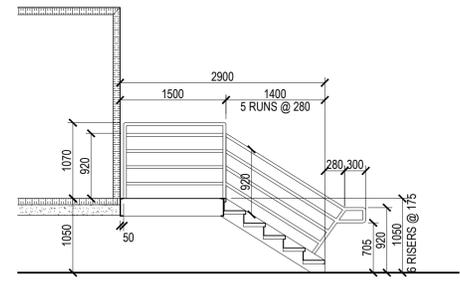
7 STAIR SECTION DETAIL AT PIL TYPICAL
