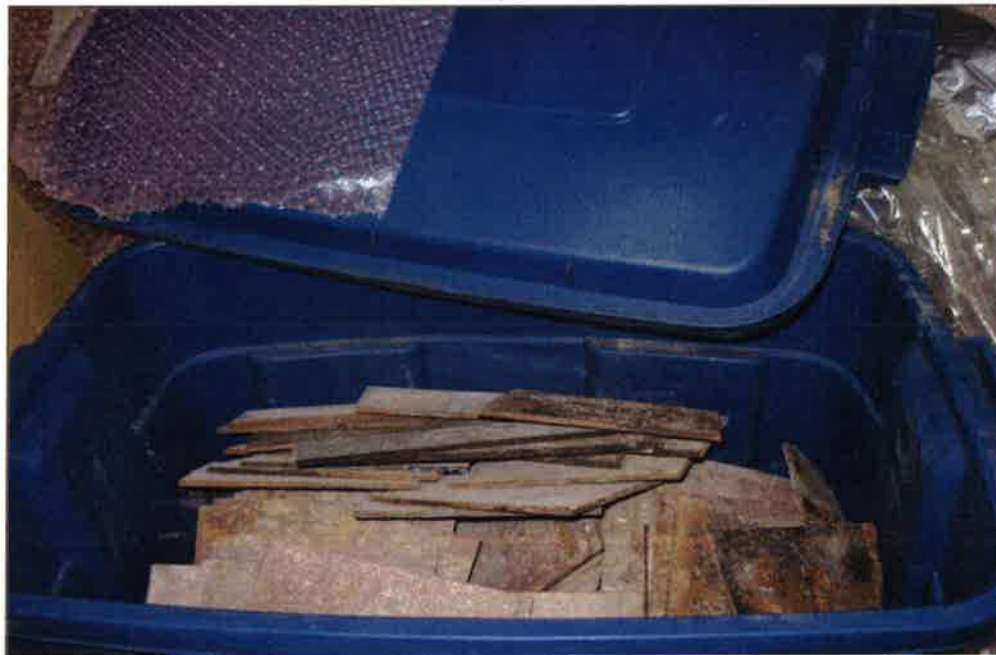
Photo 16: Asbestos containing 6"x6" brown vinyl floor tiles and 4"x4" black vinyl floor tiles. EBA sample No.Admin-004 and Admin-010. These floor tiles were visually identified on the first floor.
