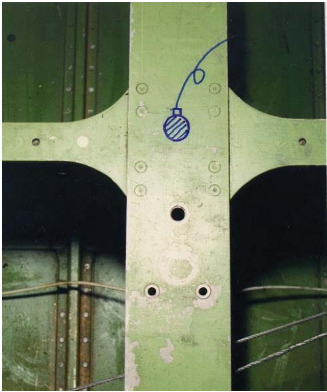
Fig. 2: Transducer Position for Calibration Scan 1 and CRT Screen Presentation
