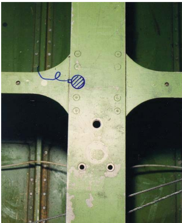
Fig. 3: Transducer Position for Calibration Scan 2 and CRT Screen Presentation
