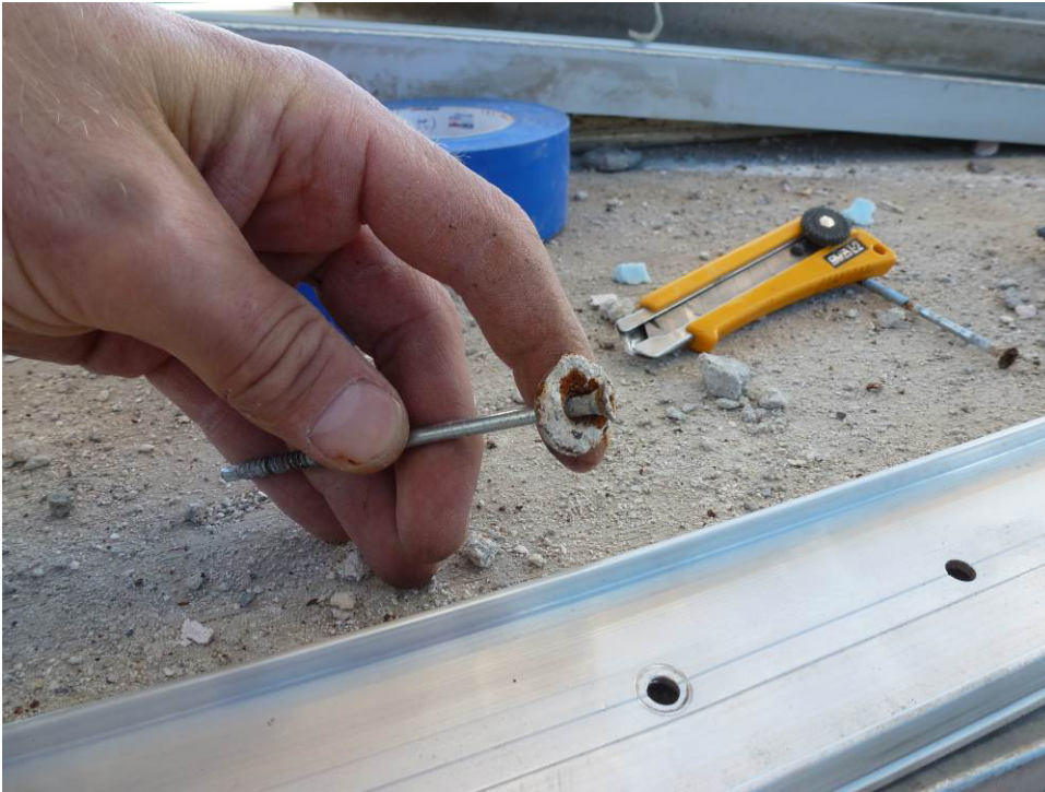
Photograph 9 – Typical Fastener Used to Secure Metal Lath into the Stud Framing Note: Corrosion.
