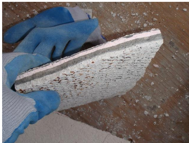
Photo 2: Cement stucco cladding.
