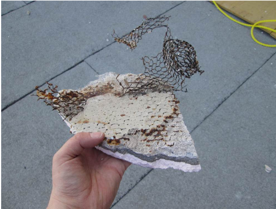
Photograph 5 – Typical Removed Stucco
