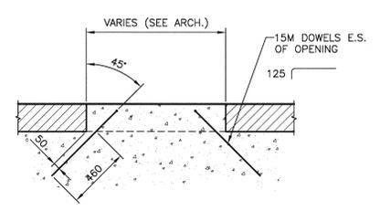
**DETAIL - TYPICAL ADD'L. REINFORCING AT DOOR OPENING**
