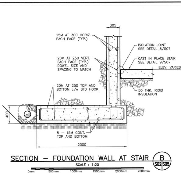
**SECTION - FOUNDATION WALL AT STAIR B**
