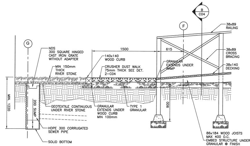
SECTION A-A: TEMPORARY RAMP AND CATCH BASIN
