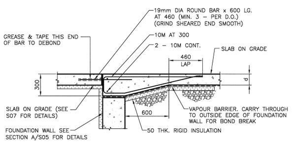
**DETAIL - TYPICAL ADD'L. REINFORCING AT DOOR OPENING**
