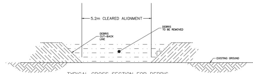
TYPICAL CROSS SECTION FOR DEBRIS AND DEADFALL CLEARING
