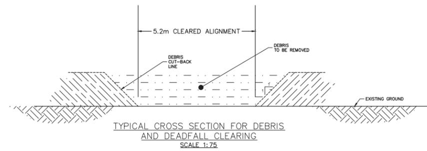
TYPICAL CROSS SECTION FOR DEBRIS AND DEADFALL CLEARING
