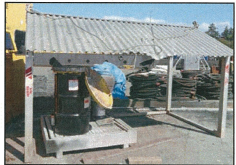
INADEQUATE: Ensure storage containers are not left open.
