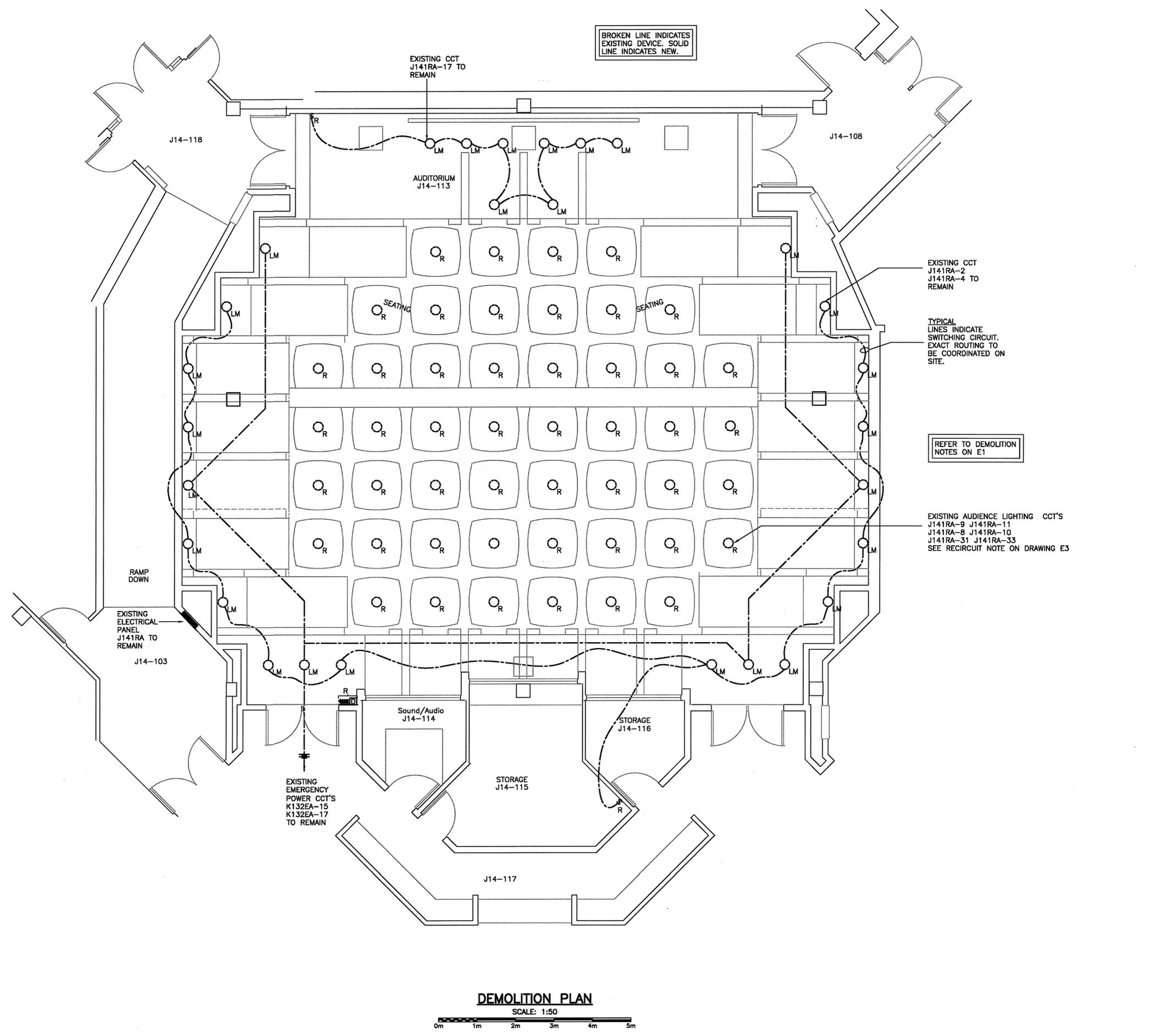
BROKEN LINE INDICATES EXISTING DEVICE, SOLID LINE INDICATES NEW.
