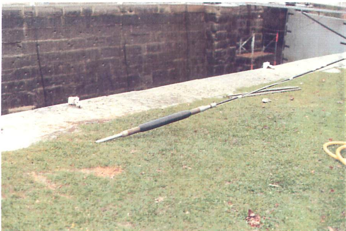
Single Inflatable Packer Assembly Showing Inflatable Packer (At Left) & Grout Pipe (Black) With Inflation Tube (White) Taped To Grout Pipe
