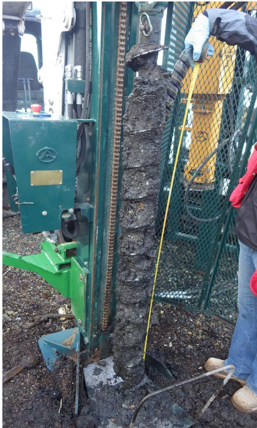
Photograph 8: silty sand on auger flight prior to collection of a bulk sample.
