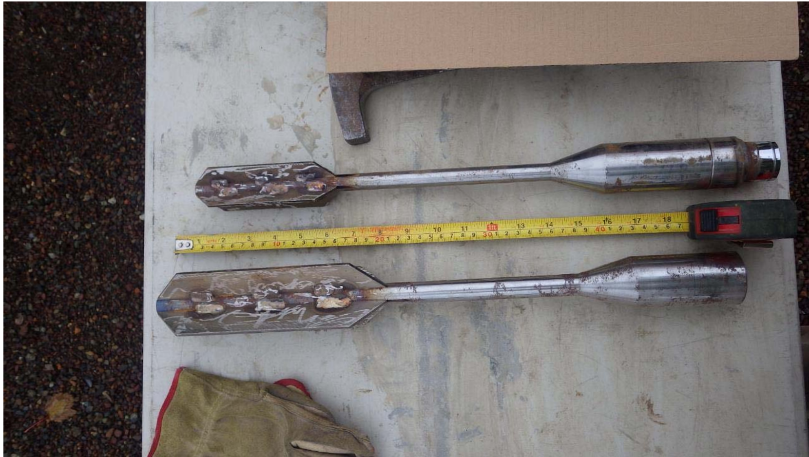
Photograph 5: Small (top) and large (bottom) shear vanes used for shear vane testing.
