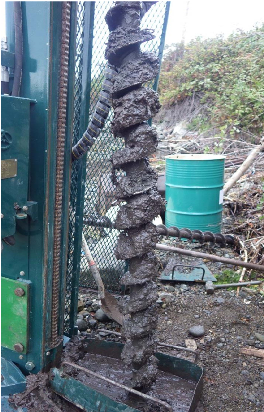
Photograph 7: Silty sand on auger flight prior to collection of a bulk sample.
