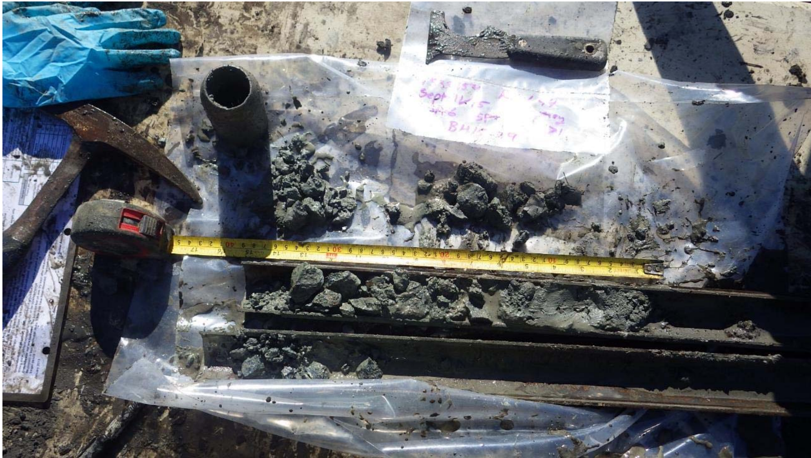
Photograph 11: Example of silty clayey sand and mechanically fractured bedrock in split spoon.
