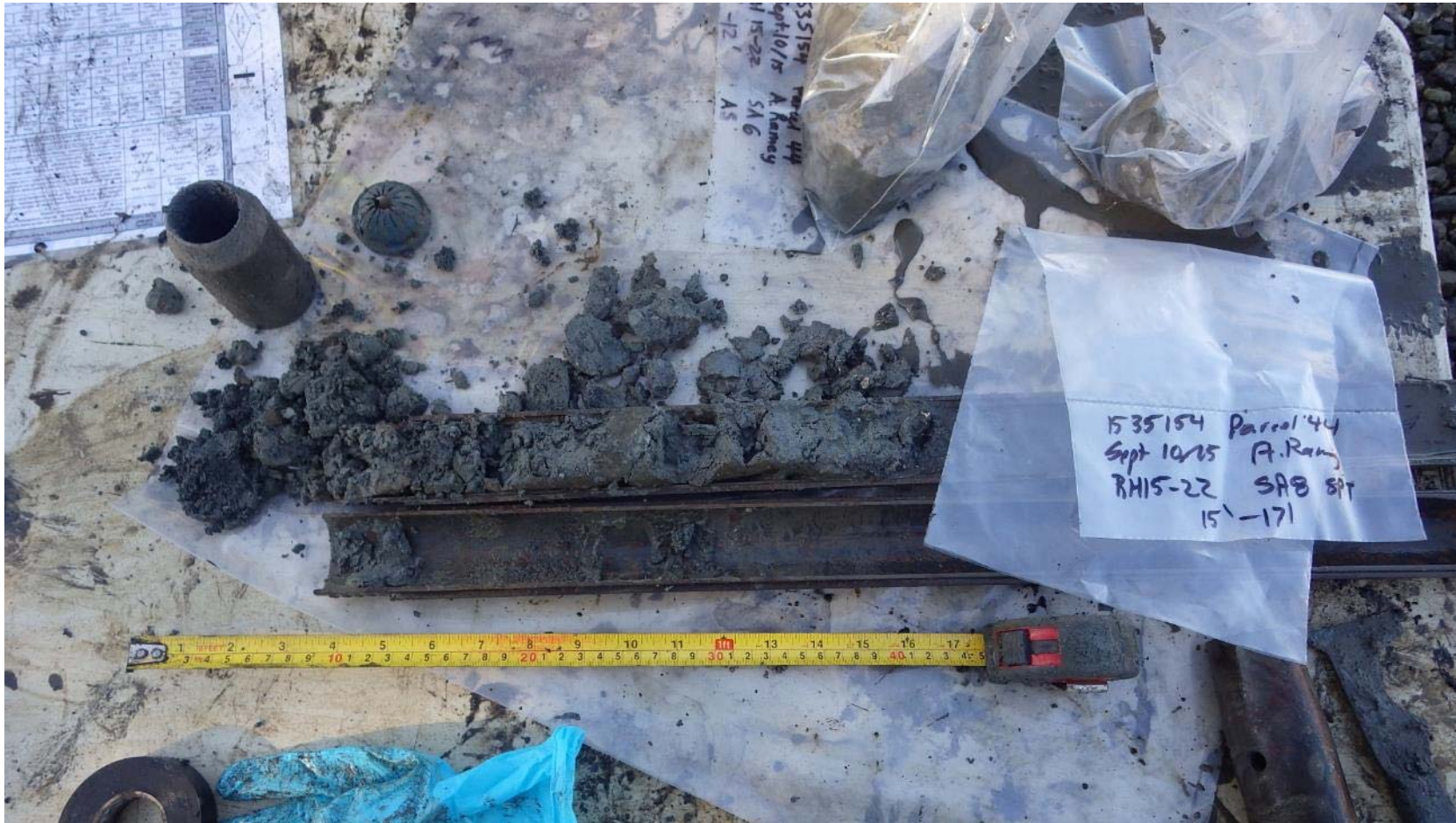
Photograph 10: Example of silty sand in split spoon.
