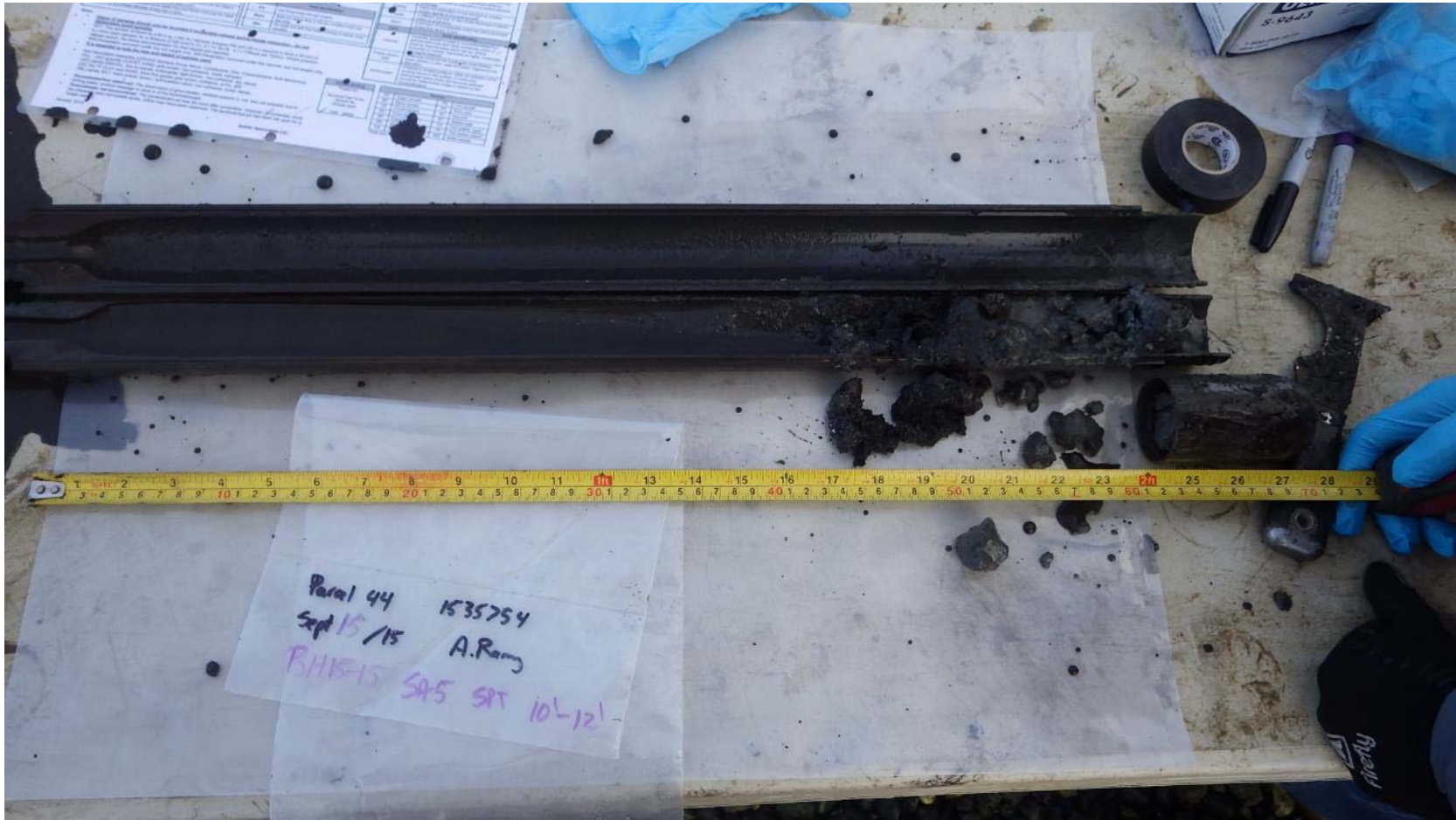
Photograph 9: Example of silty clayey sand in split spoon.
