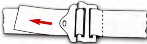
Figure 8-4 - Threading a ladderlock buckle
