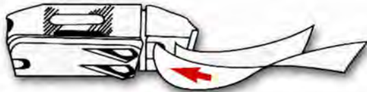
Figure 8-5 - Threading a side release buckle
