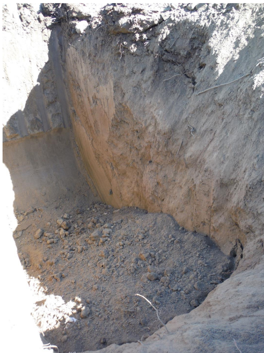
Photo 5: View of test pit TP4 showing typical native soil profile encountered in test pits surrounding the dump areas.
