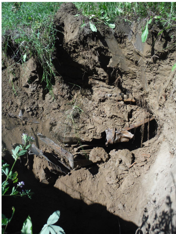
Photo 7: View of test pit TP15 completed in the north debris area. Metal encountered appeared to be a construction camp trailer.
