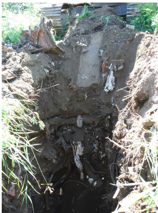
Photo 5: View of test pit TP4 showing typical native soil profile encountered in test pits surrounding the dump areas.
