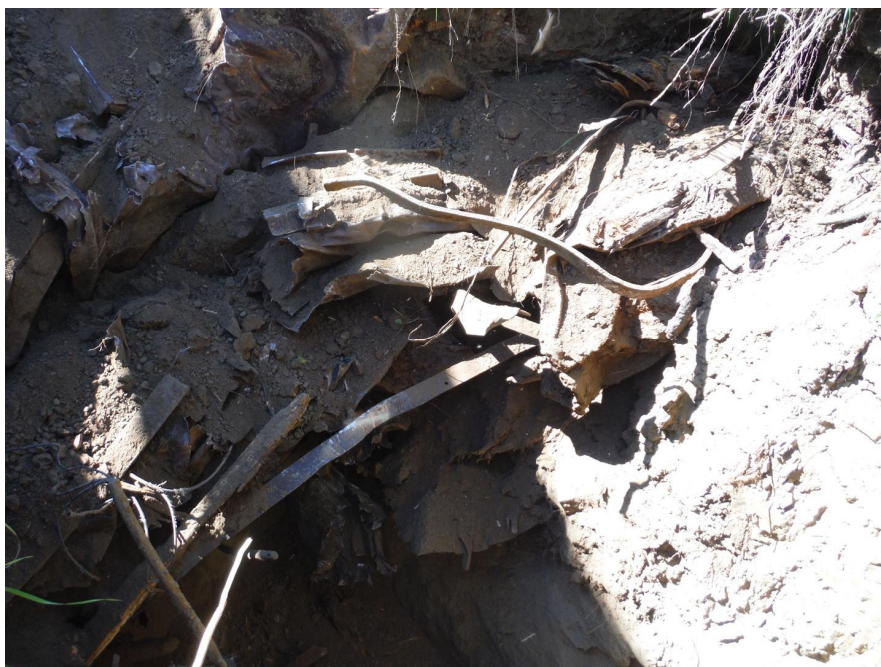
Photo 7: View of test pit TP15 completed in the north debris area. Metal encountered appeared to be a construction camp trailer.
