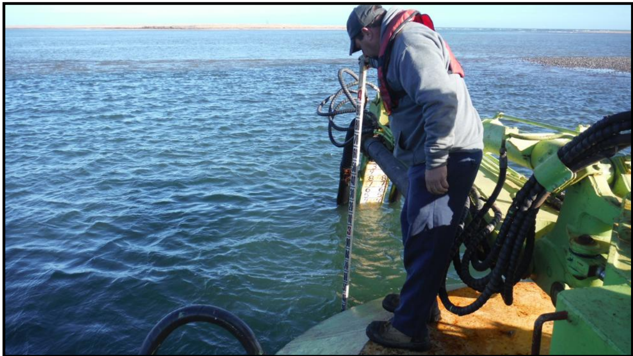
Measuring depth to ground surface. November 21, 2016.
