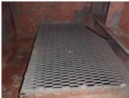
Intake screen port side. The fan and motor are directly below this screen.
