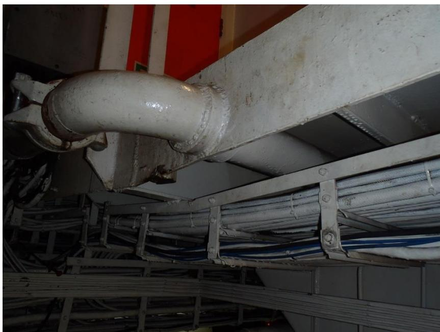
**Sewage vent pipe in port engine room extending from roust about to port sewage compartment bulkhead**
