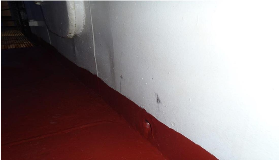
Scupper outlet from interior bulkhead on Exterior Deck
