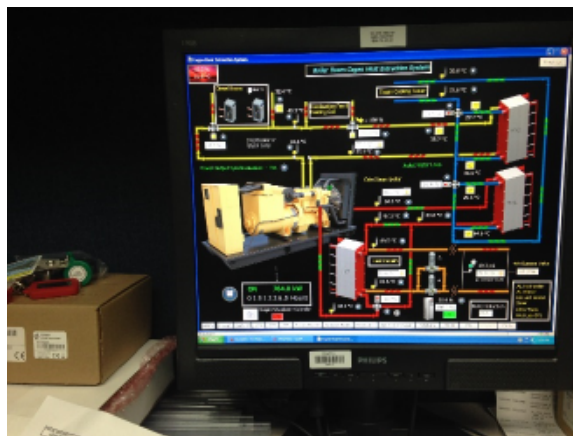
M-Figure 50 Cogen system graphics
