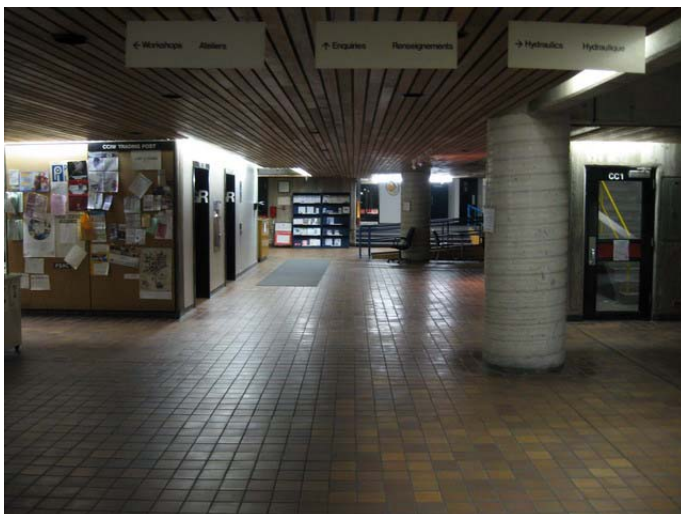
AR-123 – Exit stairwell (CC) at right, leading into 1 st floor main entrance/Mall area 'exit lobby' with excessive travel distance to exit door.
