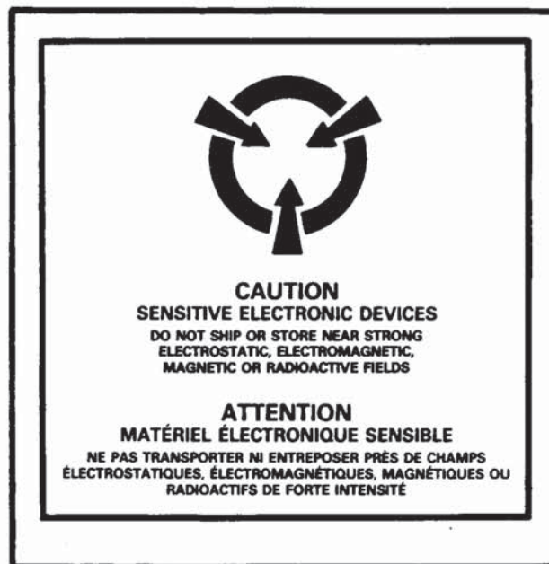
SENSITIVE ELECTRONIC DEVICE CAUTION LABEL (INTERMEDIATE AND EXTERIOR PACKS).
