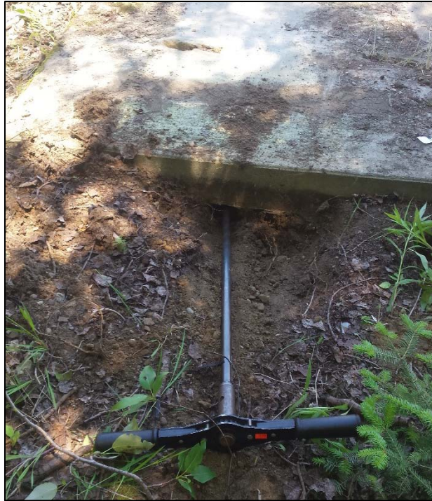
Figure 6: Hand Auguring under the concrete pad.
