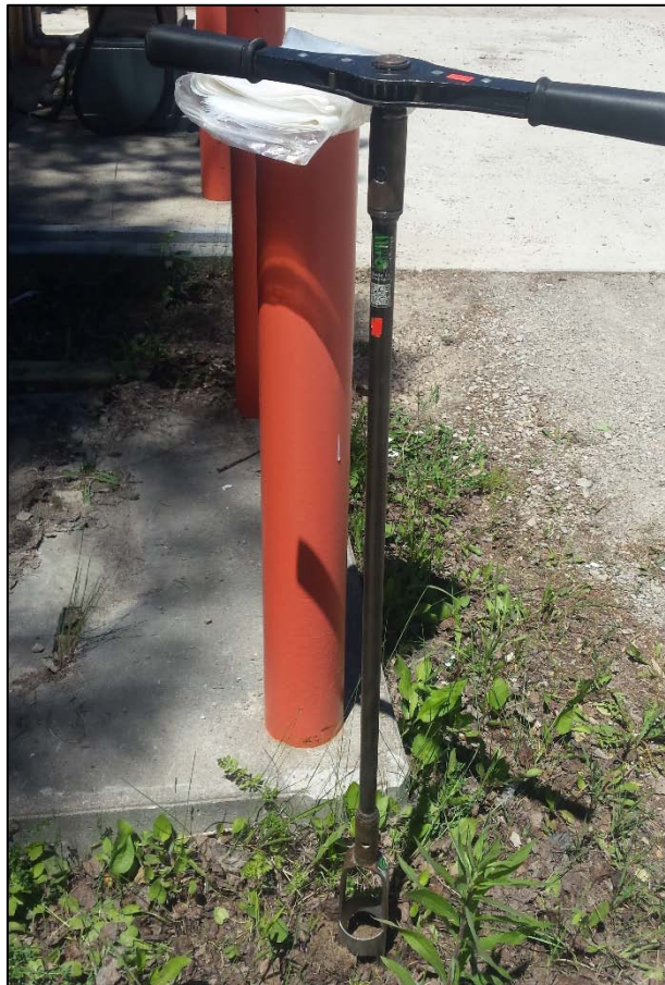
Figure 5: Hand Auguring around the perimeter of the tank pad.
