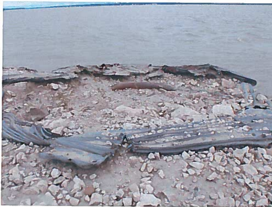
Photo 14: Failed bollard on the center of the steel caisson
