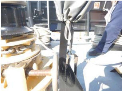
Figure 12: Guindeau et poteau à redresser Figure 13: Second angle
