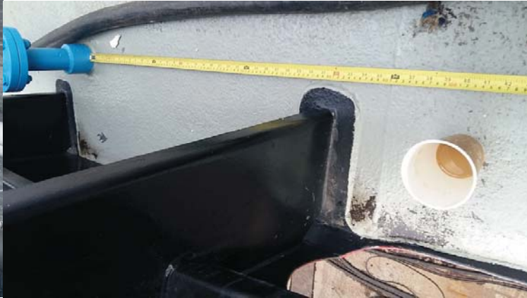
Figure 4: Distance between the end of the fresh water tank and the vent
