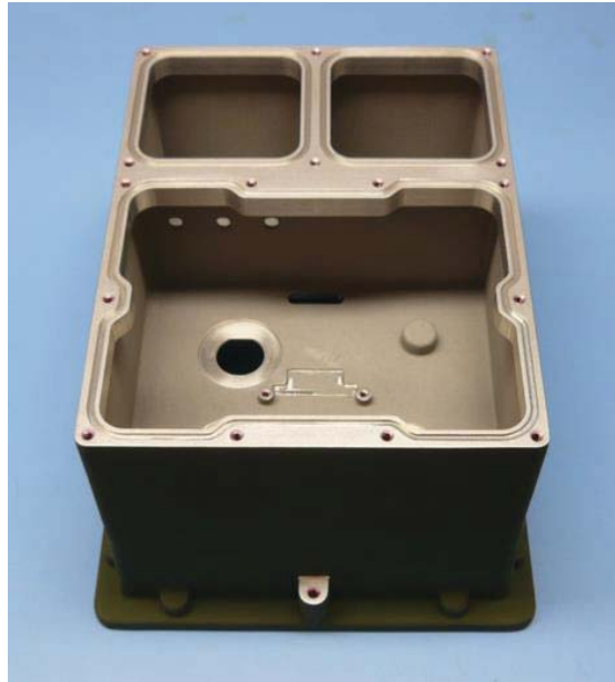
Figure A-22: Three Chambers of the VIP Mk25 Chassis
