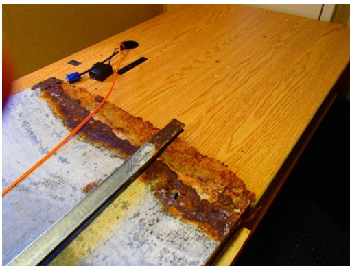
Figure 13: Corroded lower part of Joiner panel
