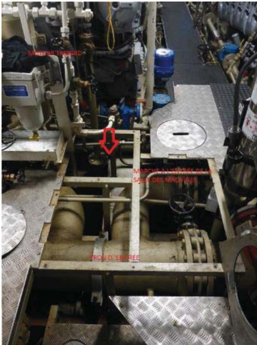
Figure 4: Location of the manhole for used Dirty oil and sludge tank (Tk 15)
