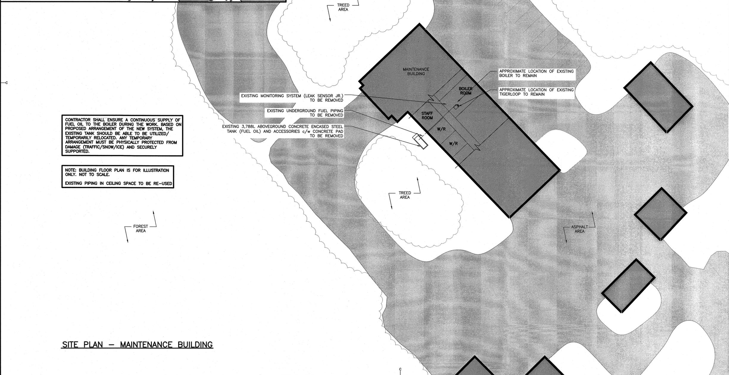
CONTRACTOR SHALL ENSURE A CONTINUOUS SUPPLY OF FUEL OIL TO THE BOILER DURING THE WORK. BASED ON PROPOSED ARRANGEMENT OF THE NEW SYSTEM, THE EXISTING TANK SHOULD BE ABLE TO BE UTILIZED/ TEMPORARILY RELOCATED. ANY TEMPORARY ARRANGEMENT MUST BE PHYSICALLY PROTECTED FROM DAMAGE (TRAFFIC/SNOW/ICE) AND SECURELY SUPPORTED.
