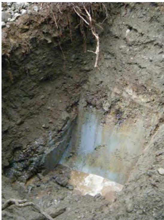
Photo 16: Granular veneer and underlying marine clay at TP16-2 (22-Nov-2016)
