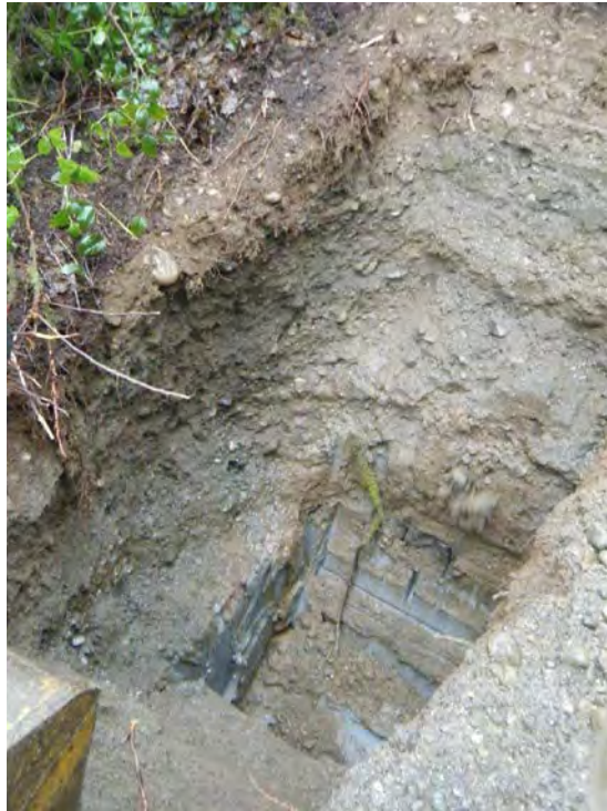
Photo 15: Granular veneer and underlying marine clay at TP16-1 (22-Nov-2016)
