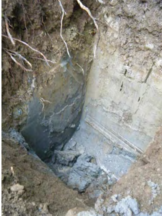
Photo 17: Marine clay with thin granular veneer at TP16-3 (22-Nov-2016)
