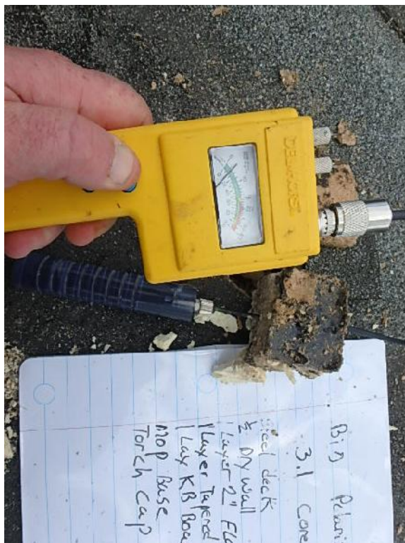
Photograph 76: Roof Area 3.1 --Roof insulation moisture test showing low levels of moisture.
