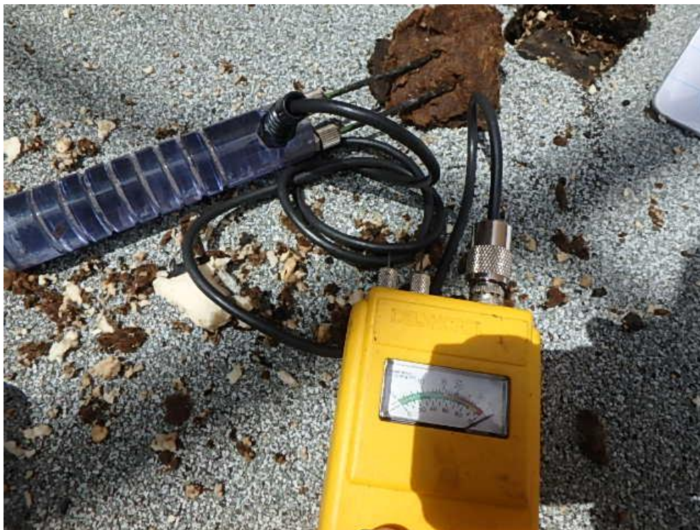
Photograph 72: Roof Area 2.2 – Roof insulation moisture test showing a completely saturated roofing system.
