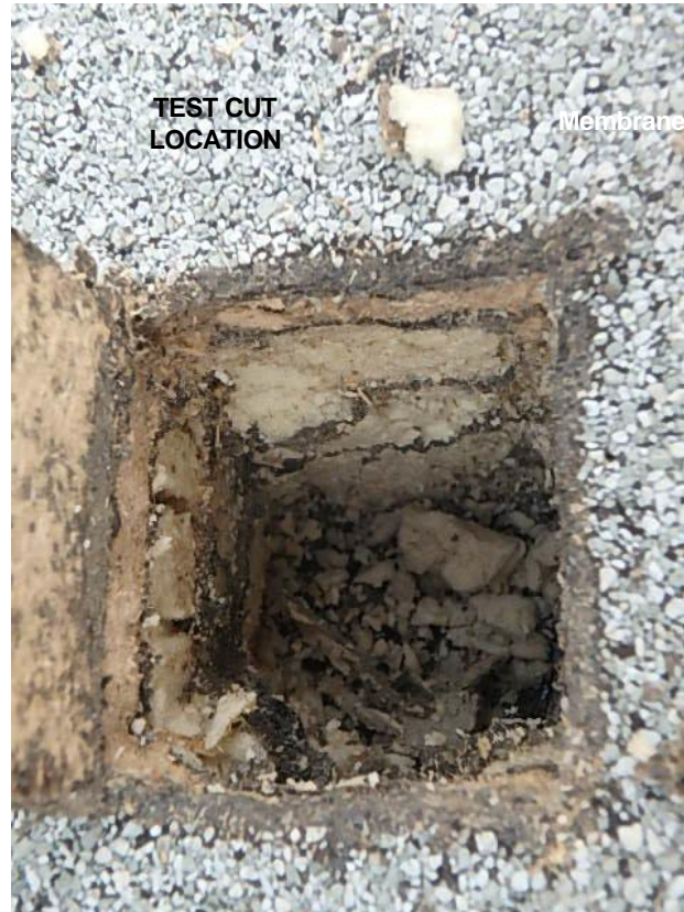
Photograph 21: Roof Area 1.1 - A core test of the roof system was conducted at a central portion of the roof.
