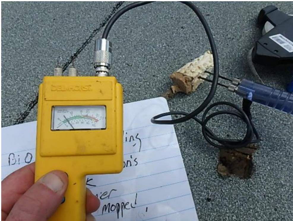
Photograph 68: Roof Area 1.1 –Roof insulation moisture test showing low levels of moisture.
