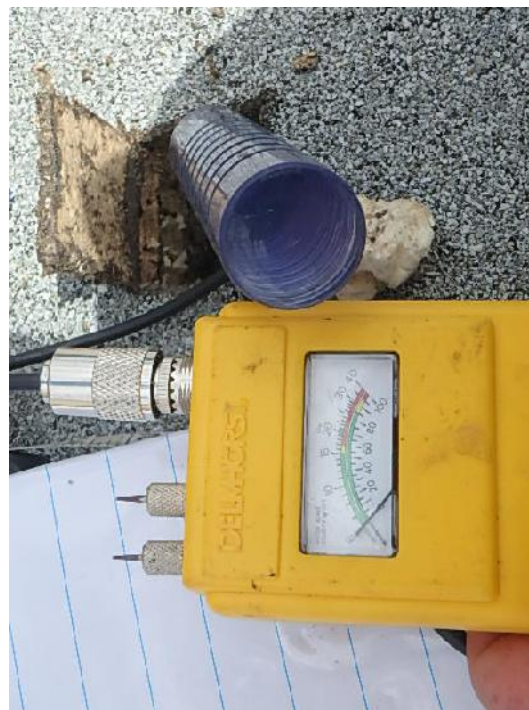
Photograph 22: Roof Area 1.1 – moisture test at core cut location.
