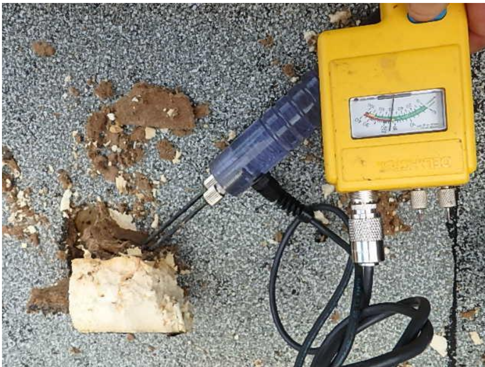
Photograph 70: Roof Area 2.1 – Roof insulation moisture test showing high levels of moisture.
