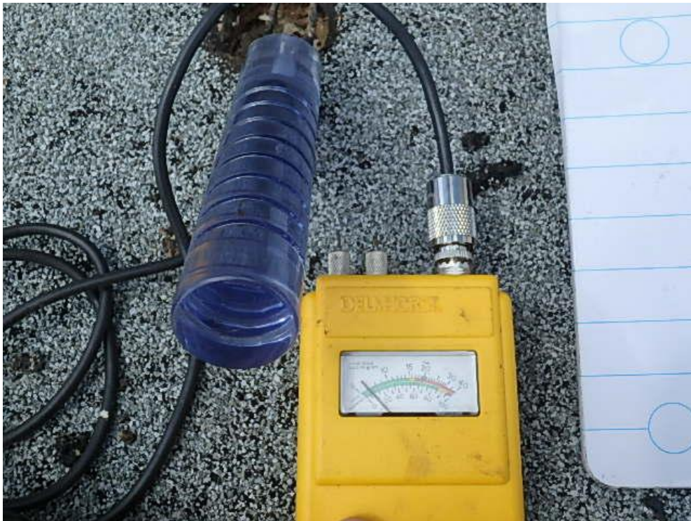
Photograph 78: Roof Area 3.3 –Roof insulation moisture test showing low levels of moisture.
