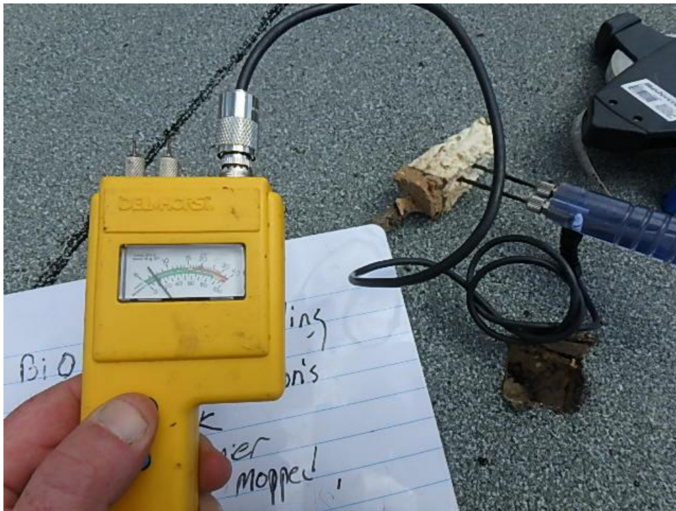
Photograph 33: Moisture testing showing a low level of moisture present in roof system.
