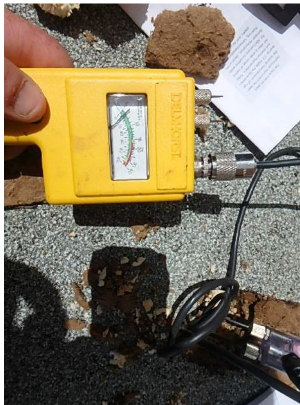
Photograph 74: Roof Area 2.3 –Roof insulation moisture test showing low levels of moisture..
