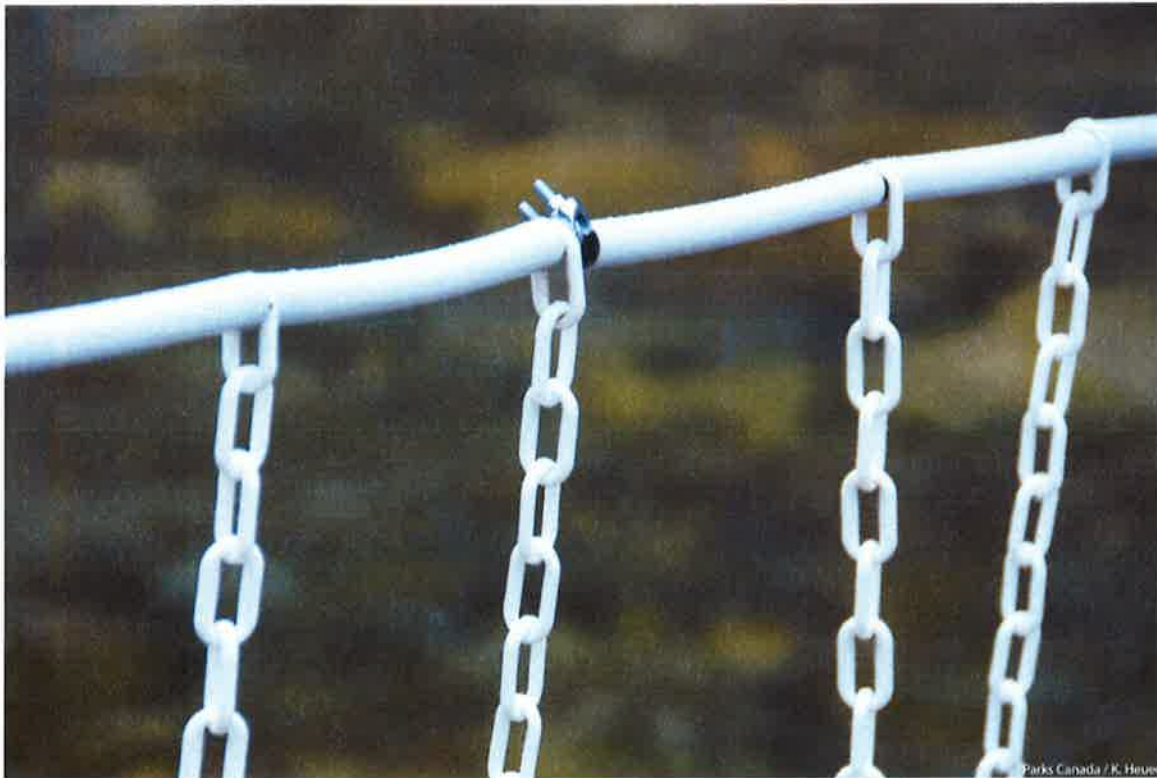
Figure 11: Close-up of plastic chain, PEX pipe spacers and cable clamps (Panther River test fence).
