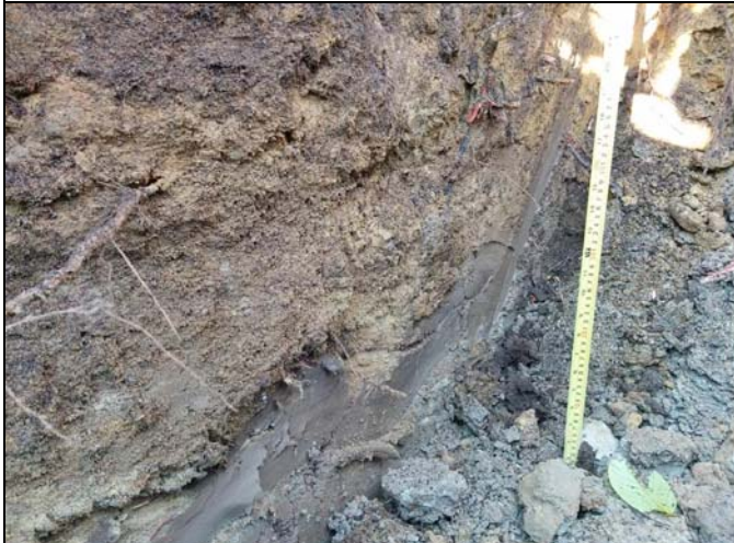
Photo 3: Sand/clay interface at depth.
