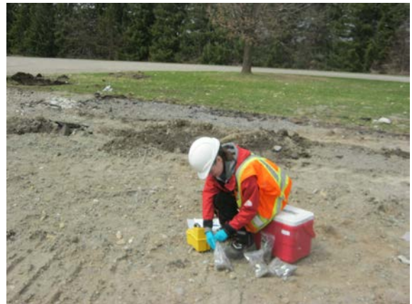
Photograph No. 6: DCS representative measuring soil vapour from collected samples using an RKI Eagle.
