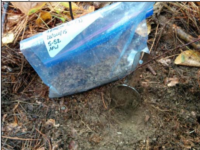
Photo 3: Sample 5-S2 soil conditions; collected ~10 m ESE of TP15-9 and ~13 m NE of TP15-8.
