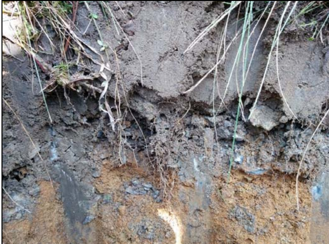
Photo 1: General view of shallow soils within the test pit, including gravel layer below topsoil.
