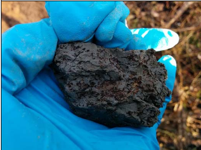
Photo 3: Mottled iron staining in stiff clay.
