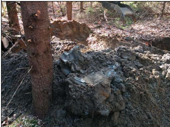
Photo 3: Sample recovered from bottom of test pit showing sand-clay interface.
