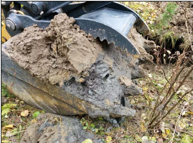
Photo 3: Fine brown sand overlying thin veneer of coarse grey sand, underlain by clay.
