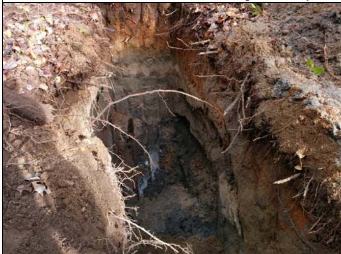
Photo 3: General view of the test pit stratigraphy to the depth of the groundwater table.
