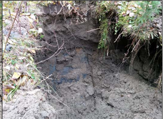
Photo 2: View of transition from fine brown sand fill to coarse grey sand; cave in due to flowing sands.
