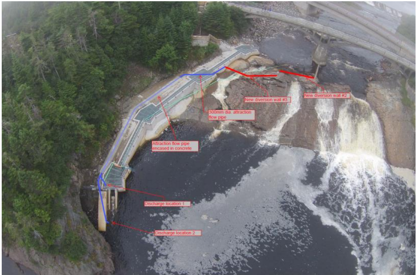
Figure 2: Drone photograph of existing fishway with components of the proposed attraction flow system sketched in.
