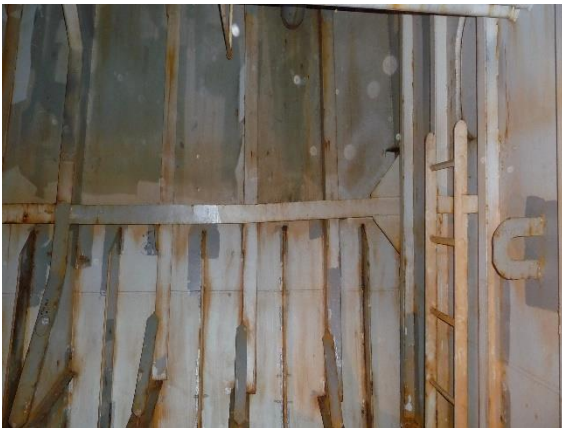
1. No 10 Port WB tank shell and framing
