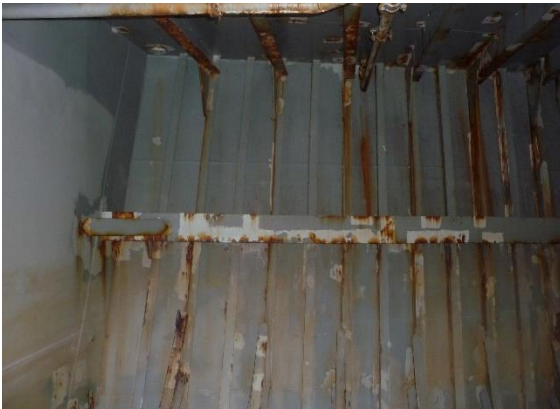
11 No 2 Stb'd WB tank shell and framing.
