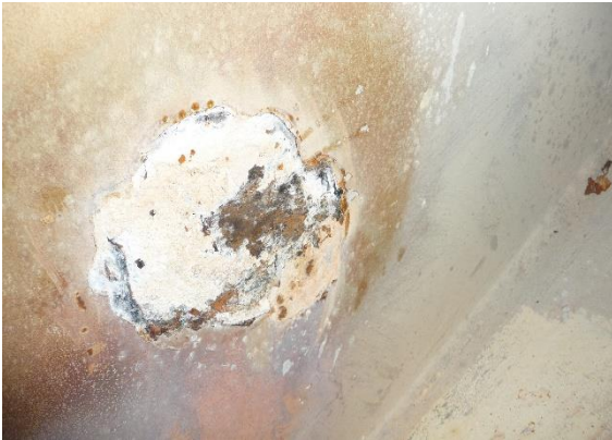
5. Photo 4 with blister removed..
