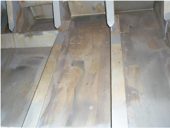
3. Side shell corrosion (typical)
