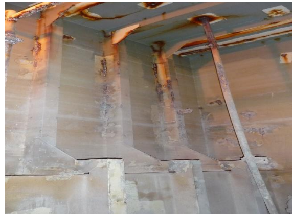
15 Stringer flat and bulkhead stiffeners..
