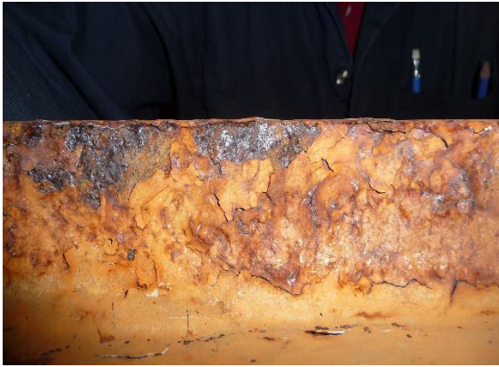
22 Corrosion under Face flat.
