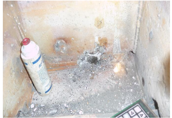
6. Severe pitting in port side girder.
