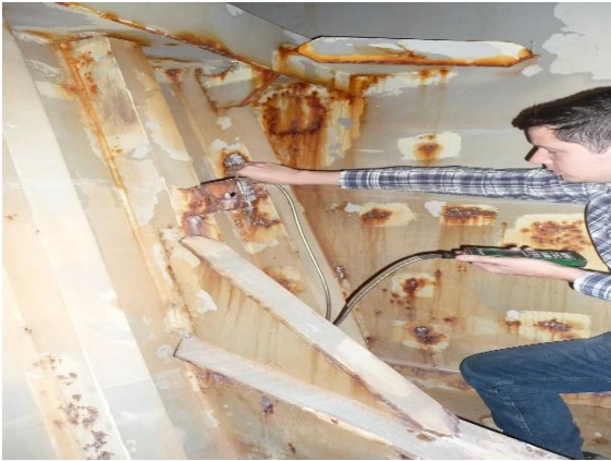
14 Typical paint deterioration and associated corrosion in way of frames.
