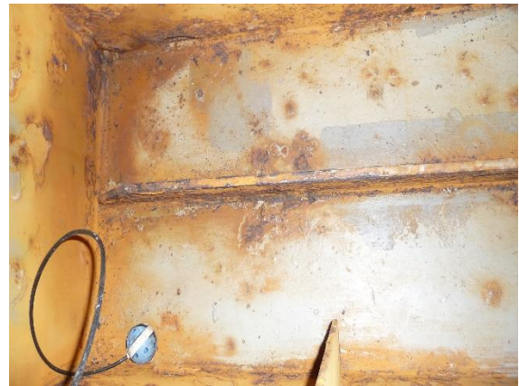
8. Typical corrosion of bottom shell and intermediate bottom transverse.
