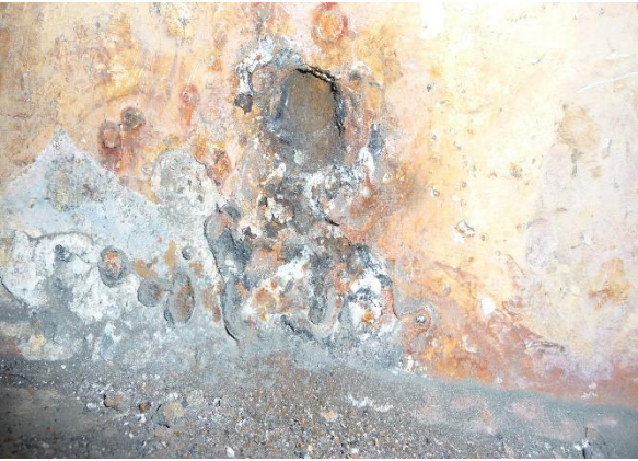
5. Severe pitting in port aft floor
