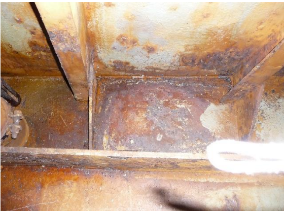
9. Corrosion in way of bulkhead.
