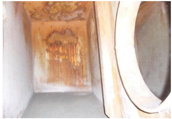
10. Typical corrosion in center tank (looking to stb'd)
