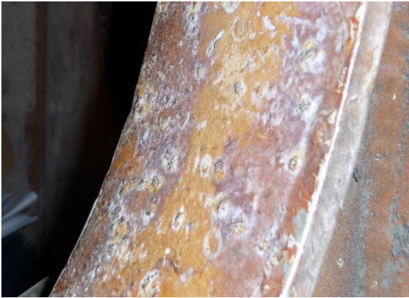
3. Corrosion in way of access coamings (typical)
