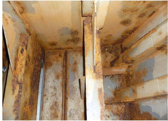
8. Typical corrosion of bottom shell and Floors.
