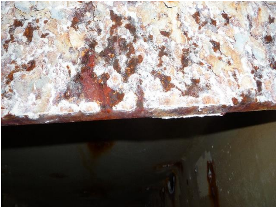
5. Badly corroded carling at tank top.
