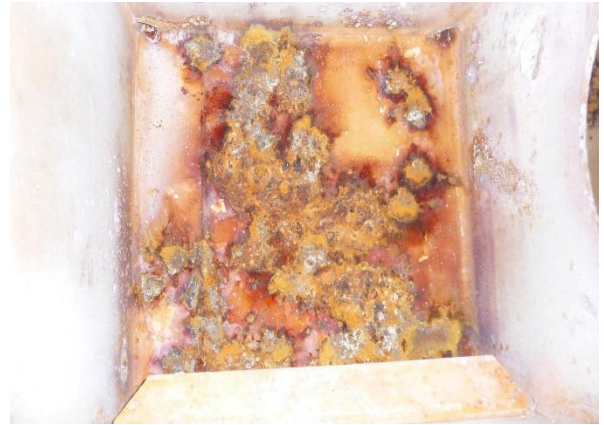
4. Typical tank top corrosion.
