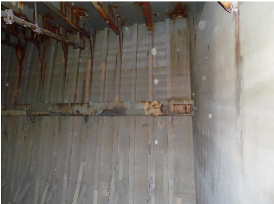
1. No 2 Port WB tank shell and framing
