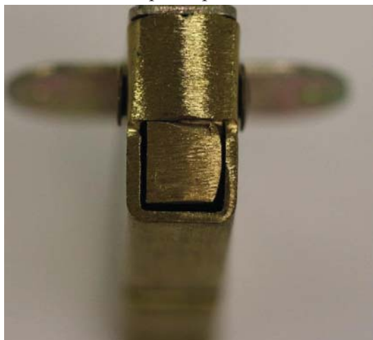
Photo # 3 Box spur – Side View
